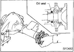
22. Install differential side shaft assembly.
