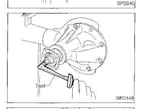
Turn drive pinion in both directions several times, and measure pinion bearing preload.
