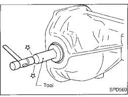
15. Apply multi-purpose grease to cavity at sealing lips of oil seal. Install side oil seal.
