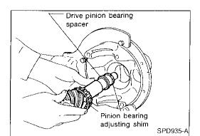
Install drive pinion bearing spacer, pinion bearing adjusting shim and drive pinion in gear carrier.
