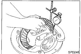
13. Tighten both right and left side bearing adjusters alternately and measure ring gear backlash and total preload at the same time. Adjust right and left side bearing adjusters by tightening them alternately so that proper ring gear backlash and total preload can be obtained.
