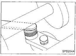
13. Select the correct standard pinion height adjusting washer thickness by using a standard gauge of 3.0 mm (0.118 in) and your J34309-101 feeler gauge. Measure the gap between the J34309-11 "R200A" pinion height adapter and the arbor.
