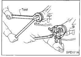
7. Loosen drive pinion nut.
