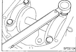
12. Install the side bearing caps and tighten the cap bolts. **Specification:**
