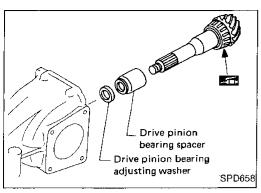
6. Place drive pinion bearing spacer, drive pinion bearing adjusting washer and drive pinion in final drive housing.
