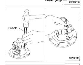
4. Install pinion mate shaft lock pin with a punch.
