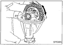
Hold companion flange steady by hand and rotate the ring gear in both directions.
