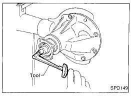
When checking preload, turn drive pinion in both directions several times to set bearing rollers.
