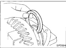
3. Put the side bearing spacer in place.
