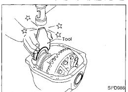
4. Using Tool, install original carrier side bearing preload shims on the carrier end, opposite the ring gear.
