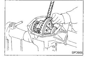
Remove differential case assembly with a pry bar.
