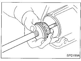
Assemble the front pinion bearing inner cone and the J34309-2 gauge anvil together with the J34309-1 gauge screw in the final drive housing. Make sure that the pinion height gauge plate, J34309-16, will turn a full 360 degrees, and tighten the two sections together by hand.
