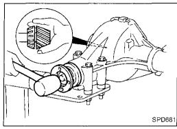
Insert companion flange into drive pinion by tapping the companion flange with a soft hammer.
