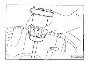
14. Remove the J34309 pinion preload shim selector tool from the final drive housing and disassemble to retrieve the pinion bearings.
