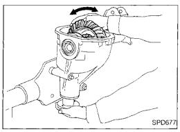
Hold companion flange steady by hand and rotate the ring gear in both directions.
