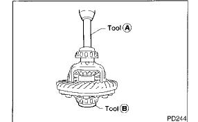
Press-fit side bearing inner cones on differential case with Tool. Tool number:
