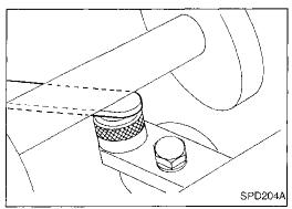
10. Select the correct standard pinion height adjusting washer thickness using a standard gauge of 2.5, 3.0, or 3.5 mm (0.098, 0.118, or 0.138 in) and your J34309-101 feeler gauge. Measure the distance between the J34309-12 "H233B" pinion height adapter and the arbor.
