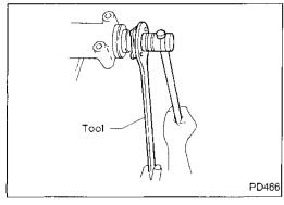
8. Tighten pinion nut to the specified torque.
