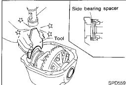
13. Drive in side bearing spacer with Tool.
