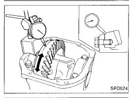
19. Check runout of ring gear with a dial indicator.
