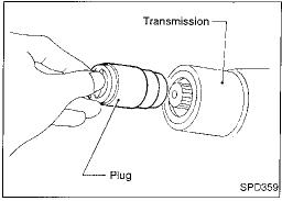
Draw out propeller shaft from transmission and plug up rear end of transmission rear extension housing.
