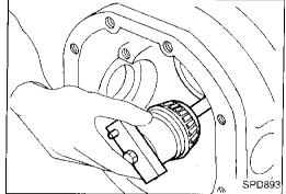
Place the pinion preload shim selector Tool, J34309-1, gauge screw assembly with the pinion rear bearing inner cone installed into the final drive housing.
