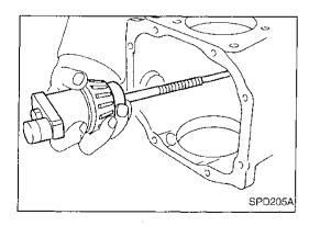
17. Remove the J34309 pinion preload shim selector tool from the final drive housing and disassemble to retrieve the pinion bearings.
