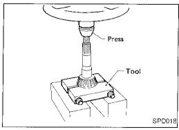
11. Remove pinion rear bearing inner cone and drive pinion adjusting washer.
