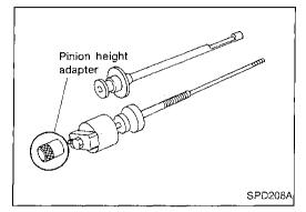
Place the J34309-12 "H233B" pinion height adapter onto the gauge plate and tighten it by hand.
