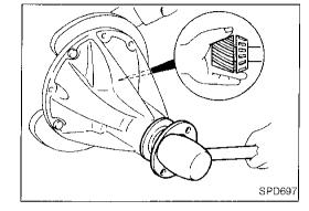
8. Tighten pinion nut to the specified torque.
