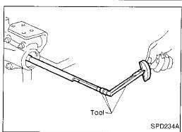
Measure the turning torque at the end of the J34309-2 gauge anvil using torque wrench J25765A.
