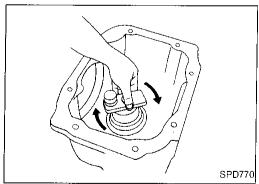
Turn the assembly several times to seat the bearings.
