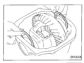
12. Insert left and right side bearing adjusting washers in place between side bearings and final drive housing.
