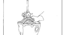
16. Measure ring gear to drive pinion backlash with a dial indicator.
