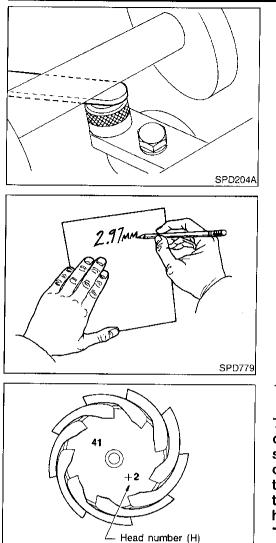
10. Select the correct standard pinion height adjusting washer thickness using a standard gauge of 2.5, 3.0, or 3.5 mm (0.098, 0.118, or 0.138 in) and your J34309-101 feeler gauge. Measure the distance between the J34309-12 "H233B" pinion height adapter and the arbor.
