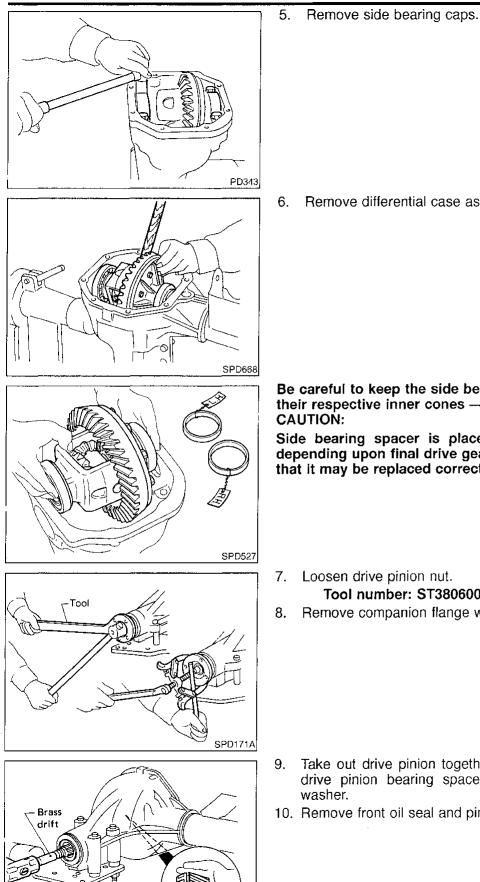
6. Remove differential case assembly with a pry bar.
