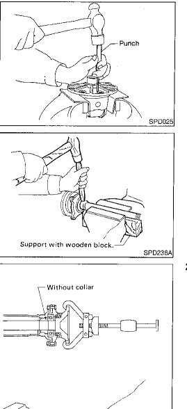
Punch off pinion mate shaft lock pin from ring gear side. 4.
