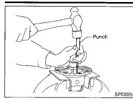
4. Drive out pinion mate shaft lock pin, with punch from ring gear side.
