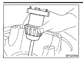
13. Remove the J34309 pinion preload shim selector tool from the GI final drive housing and disassemble to retrieve the pinion bearings.
