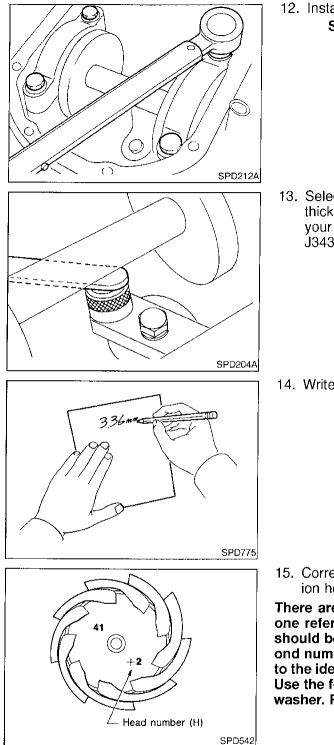
12. Install the side bearing caps and tighten the cap bolts.
