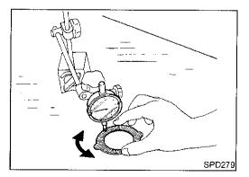
3. To test if friction disc or plate is not distorted, place it on a surface plate and rotate it by hand with indicating finger of dial gauge resting against disc or plate surface.
