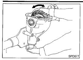
3. Hold companion flange steady by hand and rotate the ring gear in both directions.
