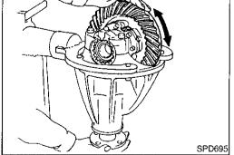
Hold companion flange steady by hand and rotate the ring gear in both directions.
