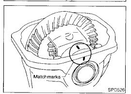
5. Install the side bearing caps in their correct locations and torque the bearing cap retaining bolts.
