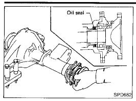
22. Install differential side shaft assembly.
