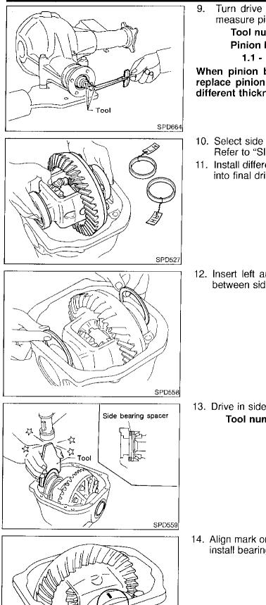
9. Turn drive pinion in both directions several revolutions, and measure pinion bearing preload.
