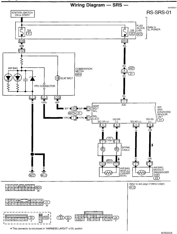
Wiring Diagram — SRS — (Cont'd)
