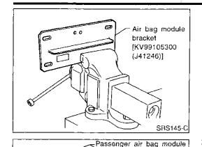
Firmly secure air bag module bracket [SST: KV99105300 (J41246)] in a vise.
