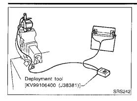
Connect red clip of deployment tool to battery positive terminal and black clip to negative terminal.
