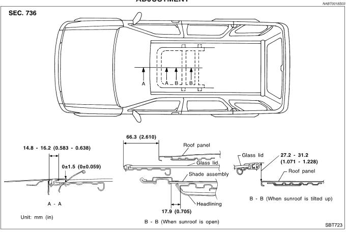
If any gap or height difference between glass lid and roof is found, check glass lid fit and adjust as follows:
