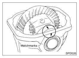
4. Put match marks on one side of side bearing cap with paint or punch to ensure that it is replaced in proper position during reassembly.
