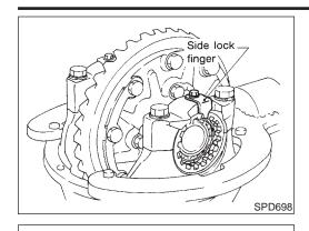
14. Tighten side bearing cap bolts.
