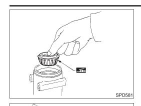
Place pinion front bearing inner cone in gear carrier.
