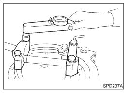
9. Install the bearing caps and torque the bolts.
