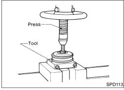
5. Remove center bearing with Tool and press. Tool number: ST30031000 (J22912-01)
