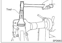
Apply multi-purpose grease to cavity at sealing lips of oil seal. Install front oil seal.
