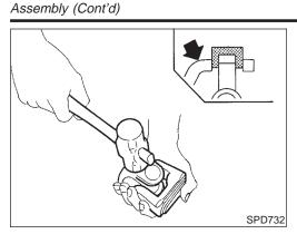
3. Adjust thrust clearance between bearing and snap ring to zero by tapping yoke.
