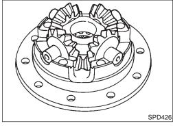
Install pinion mate gears and pinion mate thrust washers on pinion mate shaft, then install pinion mate shaft in differential case B.
