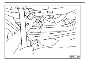
5. Apply multi-purpose grease to cavity at sealing lips of oil seal. Press front oil seal into carrier.
