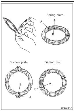
Measure frictional surfaces and projected portions of friction disc, friction plate, spring plate, and determine each part's differences to see if the specified wear limit has been exceeded.
