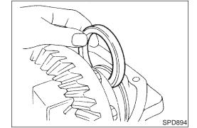
4. Using Tool, install original carrier side bearing preload shims on the carrier end, opposite the ring gear.
