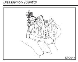
Ring gear runout
