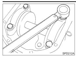
12. Install the side bearing caps and tighten the cap bolts. **Specification:**
