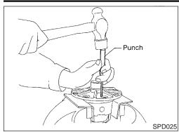
4. Punch off pinion mate shaft lock pin from ring gear side.
