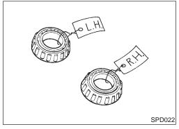
Be careful not to confuse the right and left hand parts. Keep bearing and bearing race for each side together.
