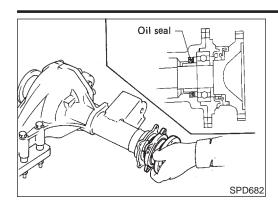
22. Install differential side shaft assembly.
