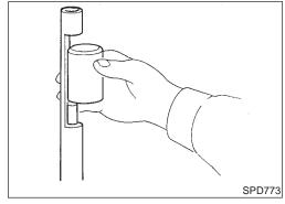
9. Select the correct thickness of pinion bearing preload adjusting washer using a standard gauge of 3.5 mm (0.138 in) and your J34309-101 feeler gauge. The exact measure you get with your gauges is the thickness of the adjusting washer required. Select the correct washer.
