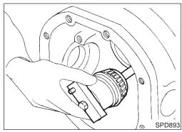
Place the pinion preload shim selector Tool, J34309-1, gauge screw assembly with the pinion rear bearing inner cone installed into the final drive housing.
