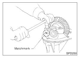
3. Remove side lock fingers and side bearing caps.
