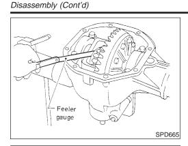
Side gear to pinion mate gear backlash
