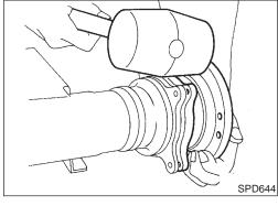
2. Remove differential side shaft assembly.
