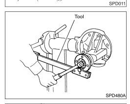
Remove drive pinion nut with Tool. Tool number: KV38108300 (J44195) Remove companion flange with puller.
