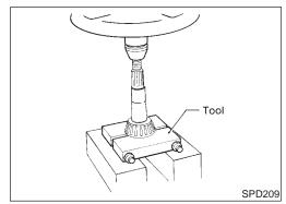
12. Remove pinion rear bearing inner cone and drive pinion height adjusting washer.
