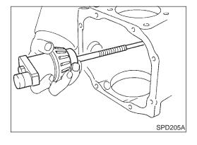
Remove the J34309 pinion preload shim selector tool from the final drive housing and disassemble to retrieve the pinion bearings.
