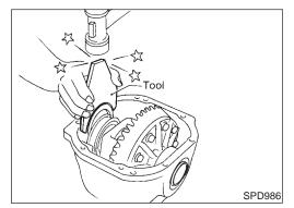
Install the side bearing caps in their correct locations and torque the bearing cap retaining bolts.
