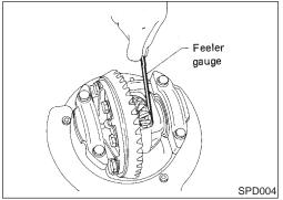
Tooth contact Check tooth contact. Refer to "TOOTH CONTACT", PD-58.
