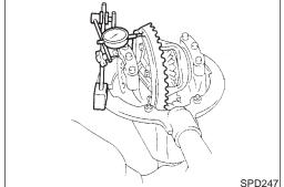
16. Check runout of ring gear with a dial indicator.
