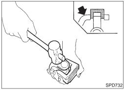
Remove pushed out journal bearing by lightly tapping yoke with a hammer, taking care not to damage journal and yoke hole.
