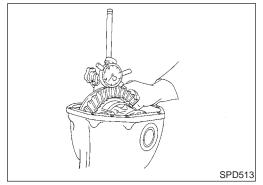
Measure ring gear to drive pinion backlash with a dial indicator.
