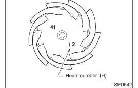
There are two numbers painted on the pinion gear. The first one refers to the pinion and ring gear as a matched set and should be the same as the number on the ring gear. The second number is the "pinion head height number", and it refers to the ideal pinion height from standard for quietest operation. Use the following chart to determine the correct pinion height washer. Refer to SDS, PD-38.
