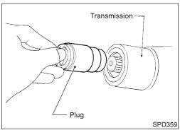
Draw out propeller shaft from transmission and plug up rear end of transmission rear extension housing.
