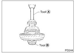
7. Press-fit side bearing inner cones on differential case with Tool.
