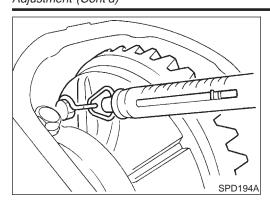
Measure the turning torque of the carrier at the ring gear retaining bolts with a spring gauge, J8129.
