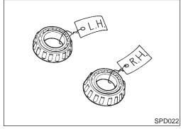
Be careful not to confuse the left and right hand parts. Keep bearing and bearing race for each side together.
