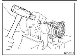
3. Remove grease seal and oil seal.
