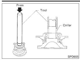
Install extension tube retainer, rear axle bearing and rear axle shaft bearing collar on differential side shaft.
