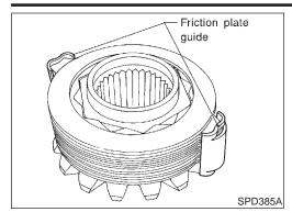
3. Install friction plate guides.
