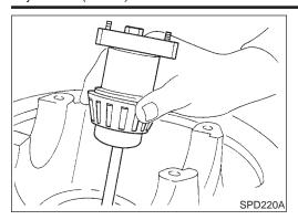
13. Remove the J34309 pinion preload shim selector tool from the final drive housing and disassemble to retrieve the pinion bearings.
