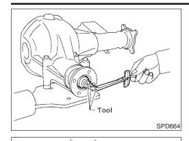
Turn drive pinion in both directions several revolutions, and measure pinion bearing preload.
