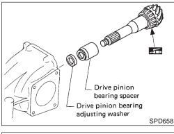
6. Place drive pinion bearing spacer, drive pinion bearing adjusting washer and drive pinion in final drive housing.
