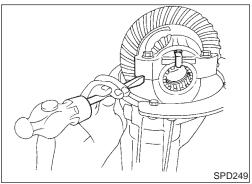
2. Put match marks on one side of side bearing cap with paint or punch to ensure that it is replaced in proper position during reassembly.
