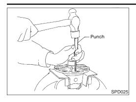
Drive out pinion mate shaft lock pin, with punch from ring gear side.
