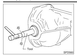
Apply multi-purpose grease to cavity at sealing lips of oil seal. Install side oil seal.
