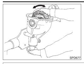
3. Hold companion flange steady by hand and rotate the ring gear in both directions.
