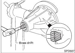
Take out drive pinion together with pinion rear bearing inner cone, drive pinion bearing spacer and pinion bearing adjusting shim.
