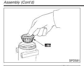
4. Place pinion front bearing inner cone in final drive housing.
