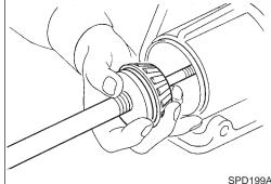
Assemble the front pinion bearing inner cone and the J34309-2 gauge anvil together with the J34309-1 gauge screw in the final drive housing. Make sure that the pinion height gauge plate, J34309-16, will turn a full 360 degrees, and tighten the two sections together by hand.
