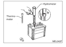
Check the charge condition of the battery. Periodically check the specific gravity of the electrolyte. Keep a close check on charge condition to prevent over-discharge.
