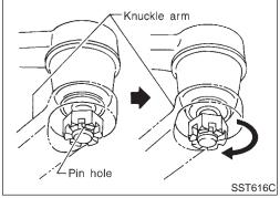
• Initially, tighten nut on tie-rod outer socket and knuckle arm to 64 to 69 N·m (6.5 to 7.0 kg-m, 47 to 51 ft-lb). Then tighten further to align nut groove with first pin hole so that cotter pin can be installed.
