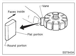
When assembling vanes to rotor, rounded surfaces of vanes must face cam ring side.
