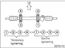
Tighten gear housing mounting bracket bolts in the order shown.
