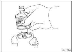
12. Install pinion assembly to rear housing. Be careful not to damage pinion oil seal.
