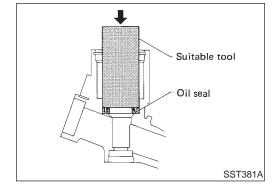
Coat seal lip of new pinion oil seal with multi-purpose grease. Install it into pinion housing of gear with a suitable tool.
