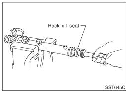
Install rack oil seal and rack bushing with rack assembly.
