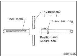
2. Using Tool, compress rack seal ring securely on rack.
