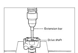
• Remove snap ring, then draw pulley shaft out. **Be careful not to drop drive shaft.**
