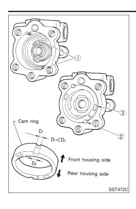
Insert pin 2 into pin groove 1 of front housing and front side plate. Then install cam ring 3 as shown at left.
