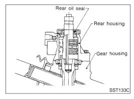
13. Apply a coat of multi-purpose grease to new rear oil seal lip before installing rear housing.
