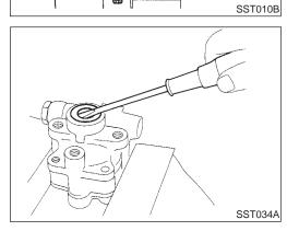
Remove connector and flow control valve with spring.
