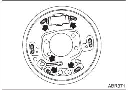
Apply brake grease to the contact areas (indicated by arrows and hatching) shown at left.
