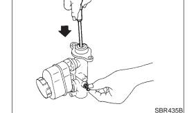
5. Install valve stopper while piston is pushed into cylinder.
