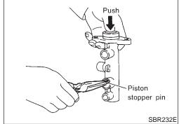
Remove piston stopper pin while piston is pushed into cylinder.
