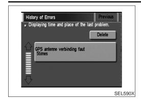
6. If trouble items are displayed with time count, repair/replace the system according to "Error history" TABLE, EL-822.
