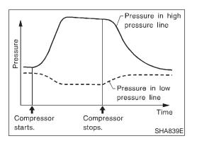
Refrigerant leaks should be checked immediately after stopping the engine. Begin with the leak detector at the compressor. The pressure on the high pressure side will gradually drop after refrigerant circulation stops and pressure on the low pressure side will gradually rise, as shown in the graph. Some leaks are more easily detected when pressure is high.
