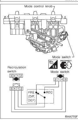
Check continuity between terminals at each switch position.
