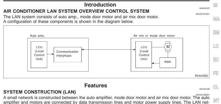
work is built through the ground circuits of the two motors. Addresses, motor opening angle signals, motor stop signals and error checking messages are all transmitted
