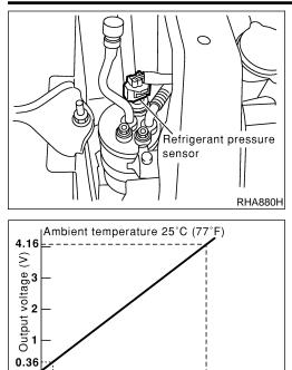
0 177 (1.8, 26) 2,746 (28, 398) (Refrigerant pressure) kPa (kg/cm², psi) Gauge pressure SHA:
