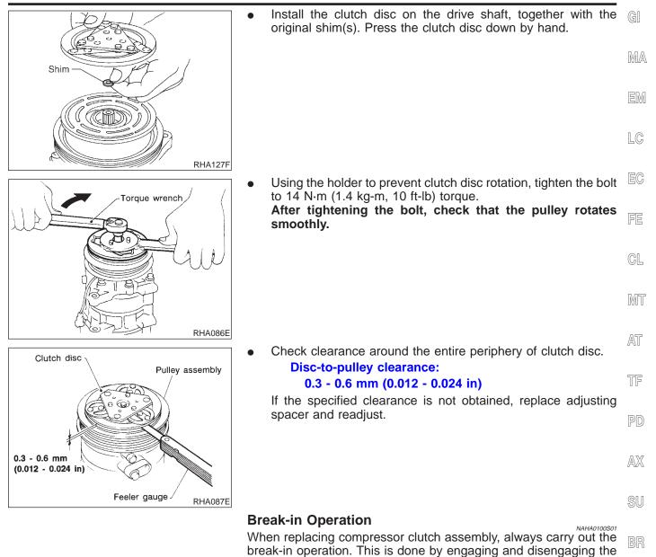
clutch about thirty times. Break-in operation raises the level of
