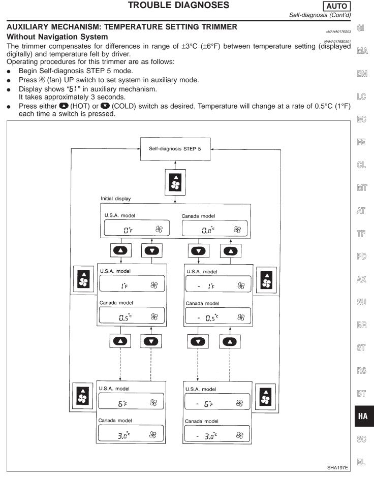
When battery cable is disconnected, trimmer operation is canceled. Temperature set becomes that of initial condition, i.e. 0°C (0°F).
