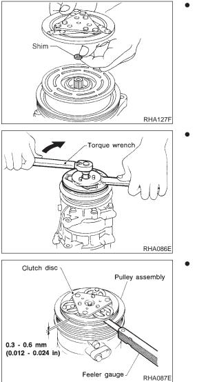
Install the clutch disc on the drive shaft, together with the original shim(s). Press the clutch disc down by hand.
