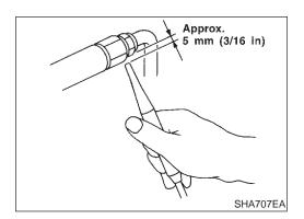
1. Position probe approximately 5 mm (3/16 in) away from point to be checked.
