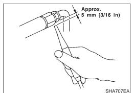
Electronic Refrigerant Leak Detector (Cont'd)
