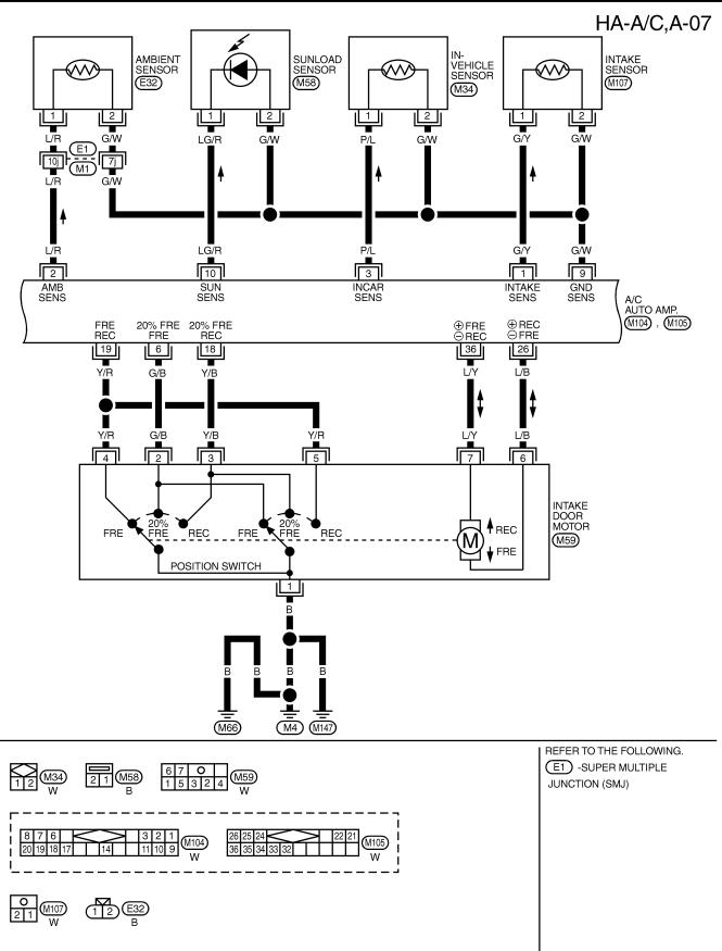
Wiring Diagram — A/C, A — (With Navigation System) (Cont'd)
