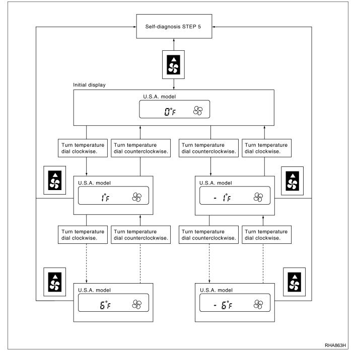
When battery cable is disconnected, trimmer operation is canceled. Temperature set becomes that of initial condition, i.e. 0°C (0°F).
