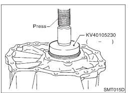
5. Set main gear bearing to front case, then press it.
