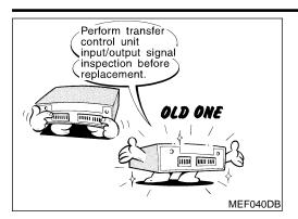
• Before replacing Transfer control unit, perform Transfer control unit input/output signal inspection and make sure whether Transfer control unit functions properly or not. (See page TF-86.)
