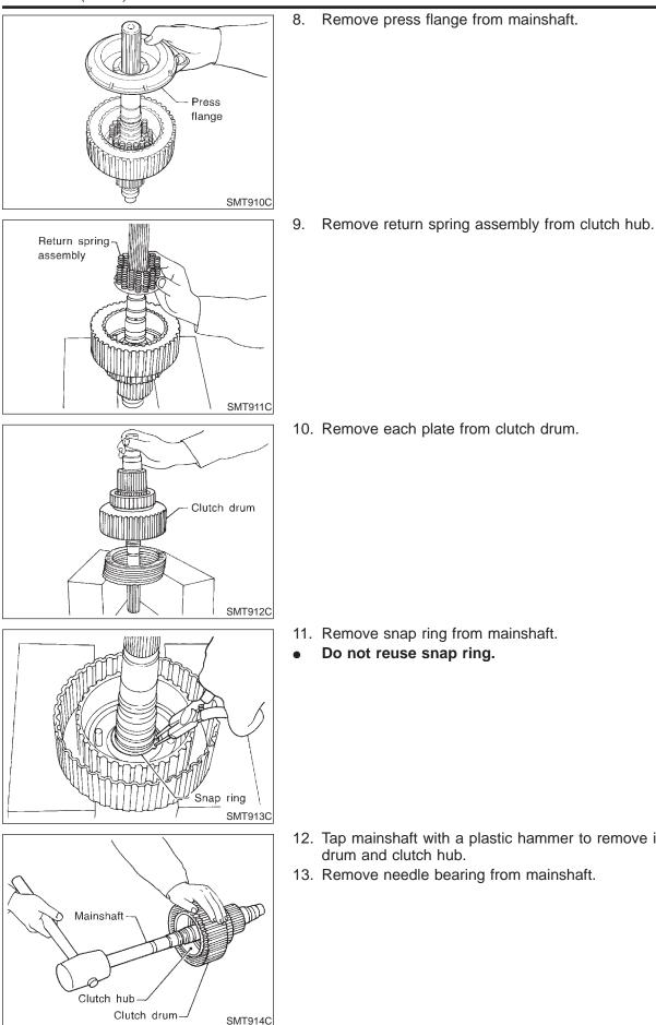
10. Remove each plate from clutch drum.
