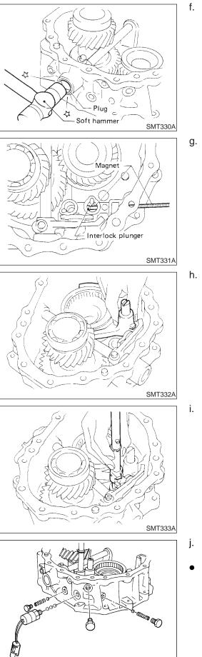
Apply sealant to plug and install it into front case. Sealant: Refer to Case Components, TF-16.
