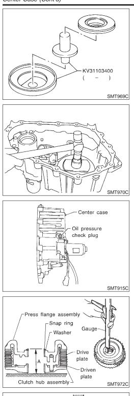
2. Set clutch piston to a clutch piston attachment (KV31103400).
