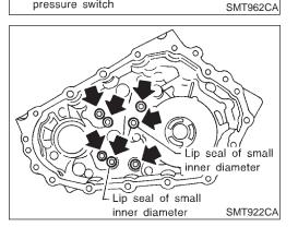
4WD solenoid valve Clutch
