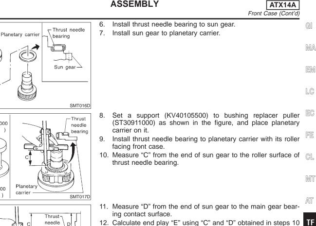
Thrust 12. Calculate end play "E" using "C" and "D" obtained in steps 10 needle С D bearing V/ Planetarycarrier Sun gear-SMT018D
