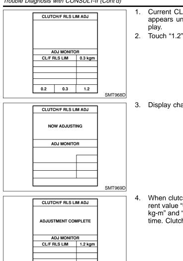
. Current CLUTCH FORCE RELEASE LIMIT value "0.3 kg-m" appears under "CONDITION SETTING" on CONSULT-II display
