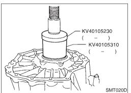
and 11. Select bearing race so that the end play becomes the standard value. PD **Calculation formula:** End play "E" = "C" - "D" Standard end play: AX 0.1 - 0.25 mm (0.0039 - 0.0098 in) **Bearing race:** SU Refer to SDS, TF-190. 13. Set planetary carrier to press in the status described in step 8. Then install the selected bearing race to planetary carrier.
