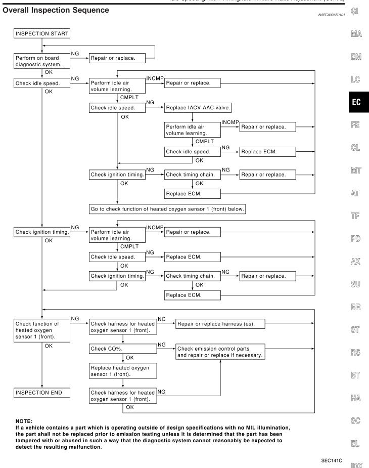
Idle Speed/Ignition Timing/Idle Mixture Ratio Adjustment (Cont'd)
