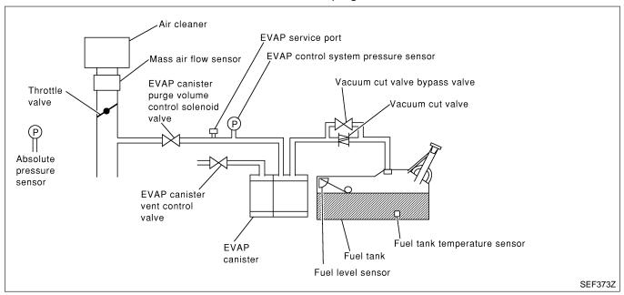
Malfunction is detected when EVAP control system has a leak, EVAP control system does not operate properly.
