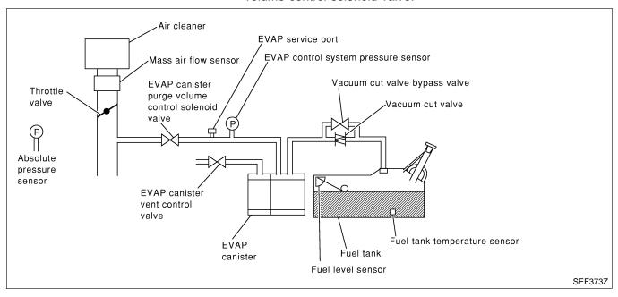
Malfunction is detected when EVAP control system has a very large leak such as fuel filler cap fell off, EVAP control system does not operate properly.
