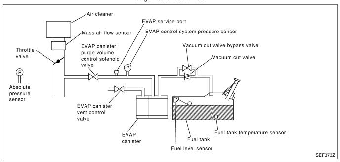
Malfunction is detected when EVAP control system has a very small leak, EVAP control system does not operate properly.
