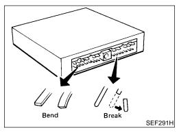
When connecting or disconnecting pin connectors into or from ECM, take care not to damage pin terminals (bend or break).
