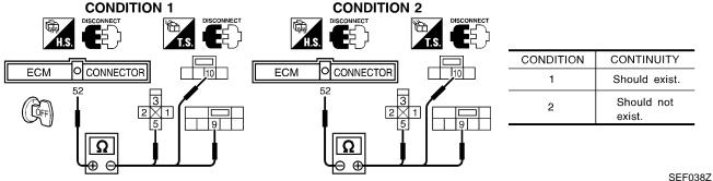
5. Check harness continuity between ECM terminal 52 and daytime light control unit terminal 5 (with autolight system for Canada) or 6 (without autolight system for Canada) under the following conditions.
