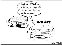
Before replacing ECM, perform "ECM Terminals and Reference Value" inspection and make sure ECM functions properly. Refer to EC-129.
