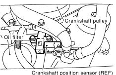
Crankshaft position sensor (REF) harness connector
