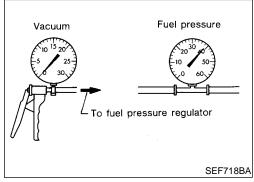
4. Start engine and read indication of fuel pressure gauge as vacuum is changed.
