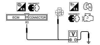
CHECK FUEL LEVEL SENSOR POWER SUPPLY CIRCUIT
