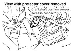
2. Check harness continuity between CKPS (POS) terminals and harness connector E132 terminals as follows.
