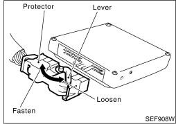
When connecting ECM harness connector, fasten it securely with a lever as far as it will go as shown at left.
