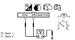
The voltage should be above 0.62V at least once during this procedure.
