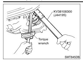
17. Install companion flange to front drive shaft, and tighten mounting nut.
