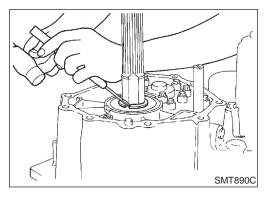
8. Remove C-rings from mainshaft bearing.
