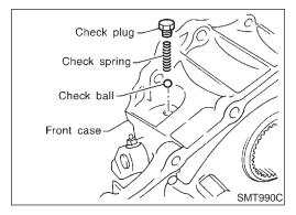
4. Remove all the liquid gasket on check plug and front case, and install check ball and check spring to front case. Apply Genuine Thread Sealant or equivalent\* to check plug, install it to front case, and tighten it to specified torque.
