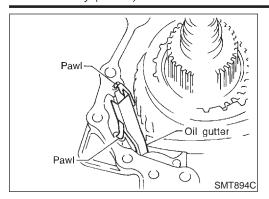
Make sure the two claws of oil gutter are securely attached to slots in center case.
