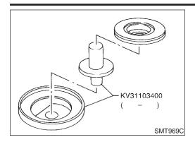
Set clutch piston to a clutch piston attachment (KV31103400).
