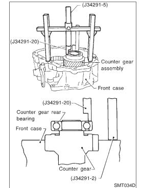
d. Place bridge, legs, gauging cylinder and gauging plunger onto machined surface of front case assembly, and allow gauging plunger to drop until it contacts counter gear rear bearing mating surface.
