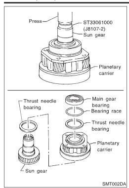
8. Set an adapter to sun gear as shown in the figure. Remove sun gear from planetary carrier. Remove main gear bearing, bearing race and thrust needle bearing (front and rear of planetary carrier) from sun gear.
