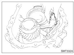
h. Install L & H shift rod and fork assembly with coupling sleeve.
