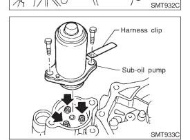
Remove sub-oil pump mounting bolts.
