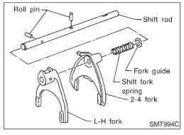
Remove L-H fork, 2-4 fork, shift fork spring and fork guide from shift rod.
