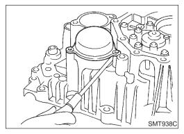
2. Insert a screwdriver as shown in the figure to remove oil filter.
