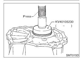
Set main gear bearing to front case, then press it.
