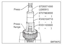
Set a drift (KV31103300), a support ring (KV40104710), a support ring (ST27863000) and a drift (ST35271000) to press flange as shown in the figure. Press drift until snap ring is out of place.
