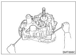
6. Insert screwdrivers as shown in the figure, and separate center case from front case. Then, remove center case by levering it up with a tire lever or the like.
