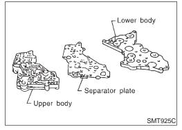
Place control valve with lower body facing up, remove two
