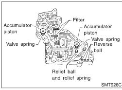
Make sure reverse balls, relief balls and relief springs, accumulator pistons, valve springs, and filters are securely installed as shown in the figure, and remove them.
