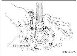
b. Install bearing retainer.
