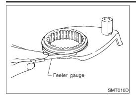
Measure clearance between shift fork and sleeve. If it is out of specification, replace it with new one.
