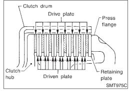
6. Install each clutch to clutch drum.
