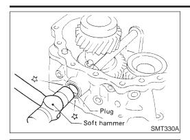
f. Apply sealant to plug and install it into front case.
