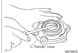
Remove oil seal from transfer cover.
