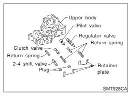
12. Remove each control valve, spring and plug.
