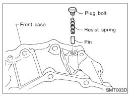
9. Remove plug bolt, then remove resist spring and pin.
