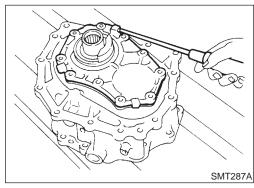
g. Remove bolts securing front case cover and then remove case.
