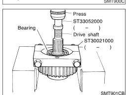
Press Bearing ST33052000 ST30021000 Drive shaft
