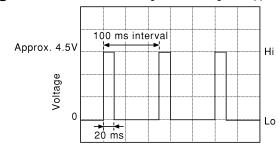
2 ABS waveform during operation
