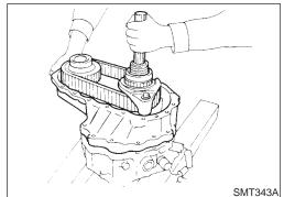
8. Install oil gutter and oil cover.
