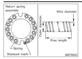
Check stamped mark shown in the figure. Then, check that free length, outer diameter and wire diameter are within specifications. If any abnormality is found, replace with new return spring assembly of the same stamped number.
