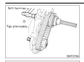
e. Remove mainshaft, front drive and drive chain as a set by tapping front end of mainshaft and front drive shaft alternately.
