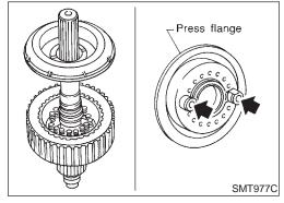
Install press flange (with the holes indicated by arrows aligned with pins of clutch hub).
