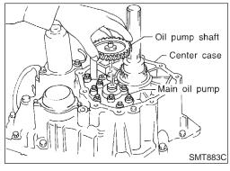
9. Fit double-flat end of oil pump shaft into slot of main oil pump and install it.
