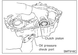
2. Apply air gradually from oil pressure check port, and remove clutch piston from center case.
