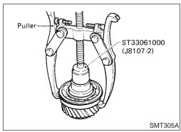
2. Pull out main gear bearing.
