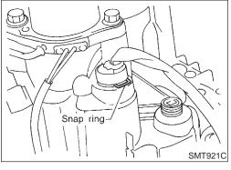
11. Secure terminal body with snap ring.
