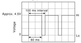
Caution: In motion, (forward to turning) changes the Hi (ON) time from 20 to 40 to 60 ms. (3) If the ABS control unit malfunctions, the terminal voltage is fixed at Hi (approximately 4.5V).
