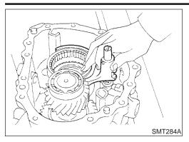
e. Remove L & H shift rod and fork assembly with coupling sleeve.
