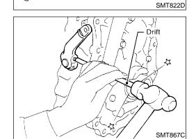
Remove lock pin of inner shift lever and drive out cross shaft with plug.
