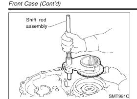
Remove shift rod components together with 2-4 sleeve and L-H sleeve.
