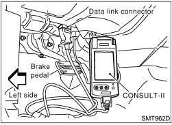
2. Connect CONSULT-II to data link connector which is located in instrument lower panel on driver side.
