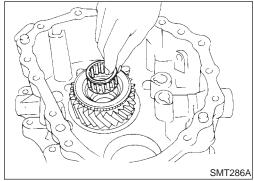
f. Remove needle bearing from main gear.
