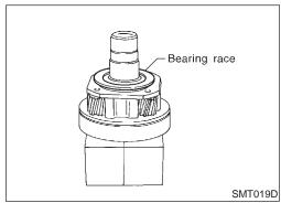
14. Install front case to planetary carrier. Set a support ring (KV40105310) and an adapter B (KV40105230) to main gear bearing inner race, then press it.
