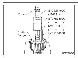
10. Pass mainshaft through snap ring. Set a drift (KV31103300), a support ring (KV40104710), a support ring (ST27863000) and a drift (ST35271000) to press flange at the position shown in the figure, and press snap ring until it fits into snap ring groove on mainshaft.
