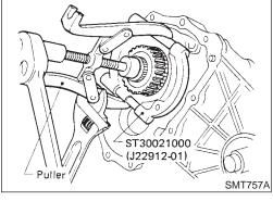
b. Pull out low gear with L & H hub.
