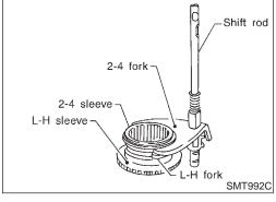
2. Install 2-4 sleeve and L-H sleeve to each fork.
