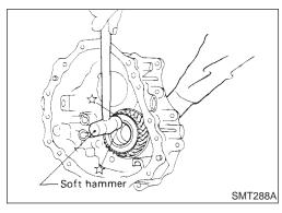
i. Remove main gear by tapping lightly.
