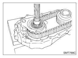
d. Make sure of the direction of the drive chain before removing it. (It must be reinstalled in the same direction.)
