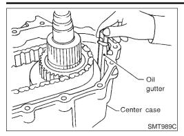
Align claw of oil gutter with center case, and install it.
