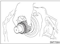
c. Remove needle bearing of low gear.
