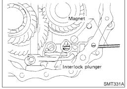
g. Insert interlock plunger into front case.
