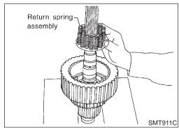
7. Align the notch of return spring assembly with the pin of clutch hub, and install it.
