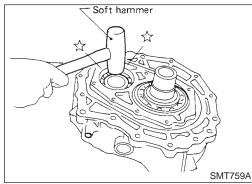
h. Remove counter gear by tapping lightly.
