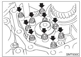
2. Install main oil pump assembly to center case assembly, and tighten bolts.
