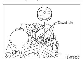
4. Align dowel pin hole and mounting bolt hole of sub-oil pump assembly with center case. Then tighten bolts.
