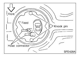
Face fuel level sensor unit as shown in the figure, and install it with knock pin on back aligned with knock pin hole on fuel tank.
