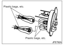
Press fuel tube and fuel level sensor unit as shown in the figure. Disconnect the joint by pushing tab and pull out fuel tube. (Return tube)
