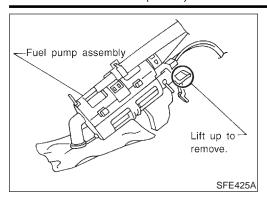
6. Remove fuel pump with bracket while lifting the pawl of the fuel pump bracket upward.
