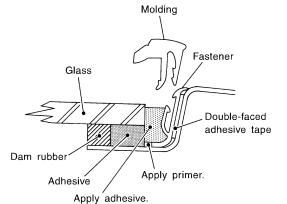
Install molding by aligning the molding mark located on center with vehicle center.
