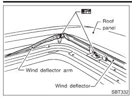
Check that wind deflector is properly retracted by hand. If it is not, remove and visually check condition. (Refer to removal procedures, BT-52.) If wind deflector is damaged, replace with new one. If wind deflector is not damaged, re-install properly.
