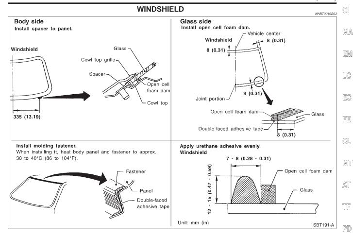
Repairing Water Leaks for Windshield
