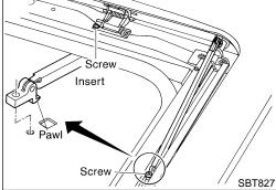
Remove screws from left and right sides of each wind deflector holder. Extract pawls through rail holes, then remove left and right sides of wind deflector holder. Remove screws from front end of sunroof unit. Extract pawls through frame holes, then remove wind deflector from frame assembly.
