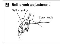
Lock door after setting door lock assembly and inside handle in position. Move bell crank in direction of arrow (shown in figure at left) to take up knob free play, and secure with bolts.
