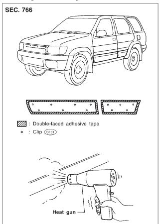
With a vehicle coated with Hard Clear Coat, use double-faced 3M adhesive tape Product No. 4210 or equivalent, after priming with 3M primer Product No. N-200 or C-100 or equivalent.
