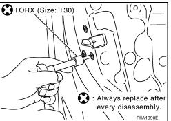
8. While pulling outside handle bracket, slide toward rear of vehicle to remove outside handle bracket and door lock assembly.
