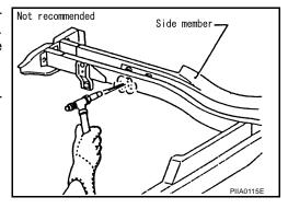
When straightening body panels, use caution in pulling any HSS panel. Because HSS is very strong, pulling may cause deformation in adjacent portions of the body. In this case, increase the number of measuring points, and carefully pull the HSS panel.
