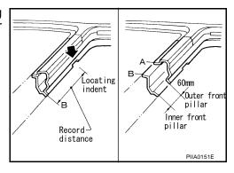
Prepare a cutting jig to make outer pillar easier to cut. Also, this will permit service part to be accurately cut at joint position.
