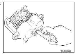
4. Using a flat-bladed screwdriver, remove piston seal from cylinder body.
