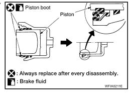
4. Insert into cylinder body by hand and insert piston boot piston-side lip into piston groove.
