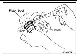
3. Apply brake fluid to piston, then install piston into cylinder body and insert piston boot side lip into groove of piston as shown.
