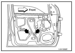
6. While holding the door window, raise it at the rear and pull the glass out of the sash toward the outside of the door.
