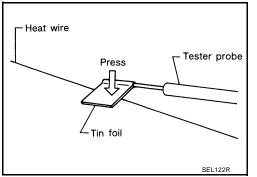
Attach probe circuit tester (in Volt range) to middle portion of each filament.
