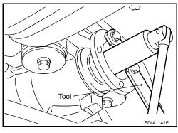
4. Remove the companion flange, using suitable tool.
