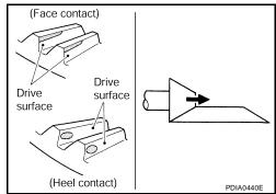
If the tooth contact is near the flank (flank contact), or near the toe (toe contact), use thinner pinion height adjusting washers to move the drive pinion farther from the drive gear.
