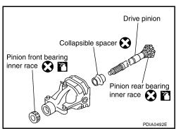
7. Press the pinion front bearing inner race to the drive pinion, using suitable spacer. Press the pinion front bearing as far as the drive pinion nut can be tightened.
