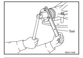
3. Put a matching mark on the end of the drive pinion in line with the matching mark B on the companion flange.
