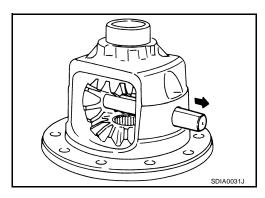
15. Turn the pinion mate gear, then remove the pinion mate gear, pinion mate thrust washer, side gear and side gear thrust washer from the differential case.
