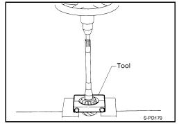
11. Remove the pinion front/rear bearing outer races by tapping them uniformly.
