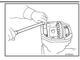
8. Lift the differential case assembly out, using suitable tool.
