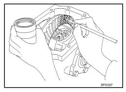
3. Rotate the drive gear back and forth several times. Check the drive pinion gear to drive gear tooth contact.
