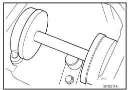
Select the correct standard pinion height adjusting washer thickness. Select by using a standard gauge of 3 mm (0.12 in) and your J-34309-101 feeler gauge. Measure the distance between the J-34309-11 pinion height adapter (including the standard gauge) and the arbor.
