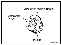
3. Remove the drive pinion lock nut, using Tool.
