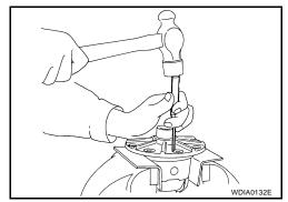
14. Remove the pinion mate shaft.
