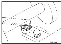
10. Write down the exact measurement (the value of feeler gauge).
