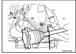
7. Place a suitable jack under the rear final drive assembly.
