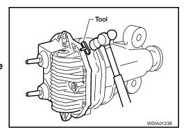
5. Mount the carrier on the Tool using two 45 mm (1.77 in) spacers.
