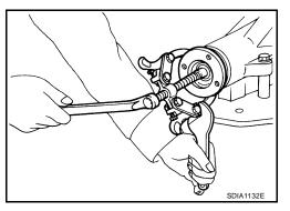
5. Press the drive pinion assembly out of the gear carrier.
