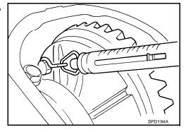
If the turning torque is outside the specification, use a thicker/ thinner side bearing adjusting washer to adjust. Refer to RFD-37, "Side Bearing Adjusting Washer".
