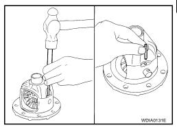
Align the matching mark of the differential case with the mark of the drive gear, then place the drive gear onto the differential case.
