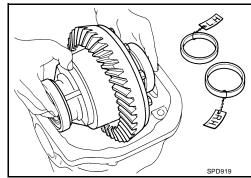
13. Insert the selected left and right side bearing adjusting washers in place between the side bearings and gear carrier.
