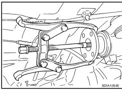
5. Remove the front oil seal, using Tool.
