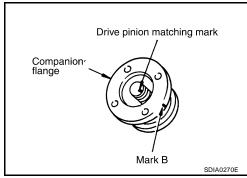
3. Install the drive pinion lock nut. Tighten to the specified torque, using Tool. Refer to <a href="RFD-16">RFD-16</a>, "COMPONENTS"</a>.
