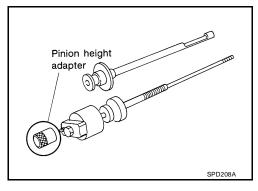
Position the side bearing discs, Tool, and arbor firmly into the side bearing bores. Install the bearing caps and tighten the bearing cap bolts to the specified torque. Refer to <a href="RFD-16">RFD-16</a>, "COM-PONENTS".
