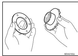
2. Install the side gears and thrust washers into the differential case.
