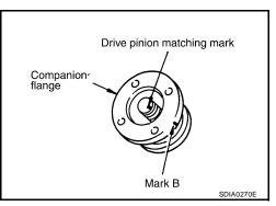
10. Apply anti-corrosive oil to the thread and seat of the drive pinion lock nut. Temporarily tighten the drive pinion lock nut to the drive pinion.
