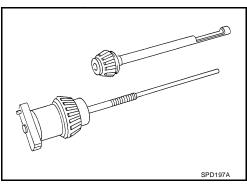
4. Assemble the pinion front bearing inner race and the J-34309-2 gauge anvil. Assemble them together with the J-34309-1 gauge screw in the gear carrier. Make sure that the pinion height gauge plate, J-34309-16, will turn a full 360 degrees. Tighten the two
