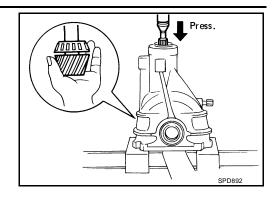
10. Remove the pinion rear bearing inner race and drive pinion height adjusting washer, using Tool.
