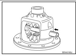
6. Drive a lock pin into the pinion mate shaft. Make sure the lock pin is flush with the differential case.
