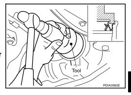
2. Align the matching mark of the drive pinion with the matching mark B of the companion flange, then install the companion flange.
