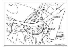
4. Remove the side oil seal, using suitable tool.
