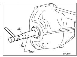
17. Check and adjust the drive gear runout, tooth contact, drive gear to drive pinion backlash, and total pre-load torque. Refer to <a href="RFD-17">RFD-17</a>, "Total Preload Torque"</a>, . RFD-17, "Total Preload Torque".
