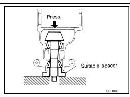
8. Install the front oil seal, using Tool.
