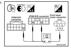
4. Check continuity between IPDM E/R harness connector terminals and ground.
