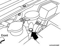
Washer fluid level sensor connector
