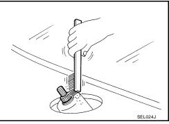
2. Lift the wiper blade up, then rest it onto glass surface to set clearance "L1" and "L2" as illustrated.
