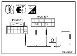
5. Check continuity between IPDM E/R harness connector terminal and ground.
