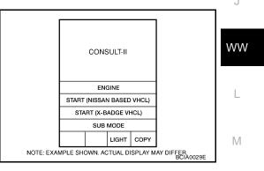
Touch "IPDM E/R" on "SELECT SYSTEM" screen. If "IPDM E/R" is not displayed, go to <u>GI-39, "CONSULT-II Data</u> <u>Link Connector (DLC) Circuit"</u>.
