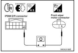
4. Check continuity between IPDM E/R harness connector E122 terminal 43 and ground.
