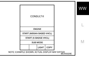
3. Touch "BCM" on the "SELECT SYSTEM" screen. If "BCM" is not indicated, go to <u>GI-39, "CONSULT-II Data Link</u> <u>Connector (DLC) Circuit"</u>.
