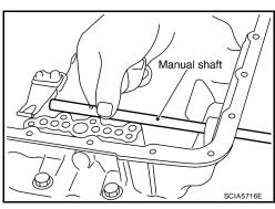
65. Remove manual shaft oil seals using suitable tool.
