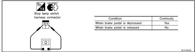
Check stop lamp switch after adjusting brake pedal — refer to BR-6, "BRAKE PEDAL".
