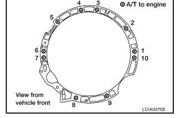
Align the positions of bolts for drive plate with those of the torque converter, and temporarily tighten the bolts. Then, tighten the bolts with the specified torque.
