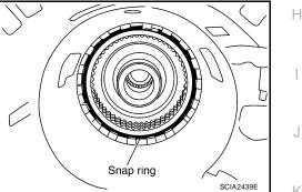
22. Measure clearance between retaining plate and snap ring. If not within specified clearance, select proper retaining plate.
