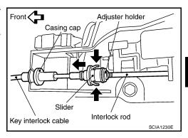
3. Remove holder from key cylinder and remove key interlock cable.
