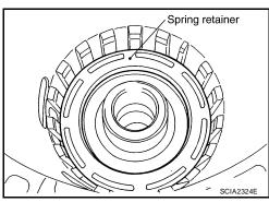
56. Remove seal rings from drum support.
