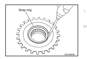
b. Remove 1st one-way clutch from rear sun gear.
