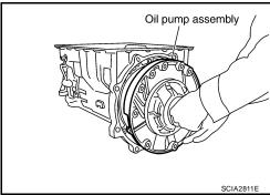
4. Apply recommended sealant (Genuine RTV Silicone Sealant or equivalent. Refer to GI-47, "Recommended Chemical Products and Sealants" .) to oil pump assembly as shown.
