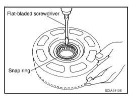
2. Remove 3rd one-way clutch from front sun gear.
