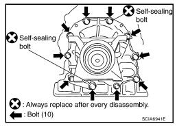
Tap rear extension assembly with soft hammer.
