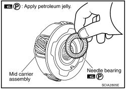
44. Install mid carrier assembly in rear carrier assembly.
