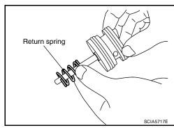
10. Install servo assembly in transmission case.
