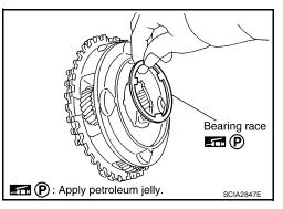
Remove needle bearing from front carrier assembly.
