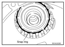
55. Remove spring retainer and return spring from transmission case.
