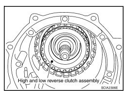
37. Align the drive plate using suitable tool.
