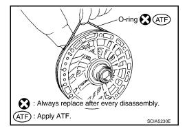
2. Install O-ring to oil pump housing.
