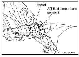
f. Install A/T fluid temperature sensor 2 (with bracket) in control valve with TCM and tighten bolt to specified torque.
