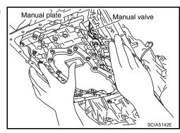
8. Install bolts A, B and C in control valve with TCM.
