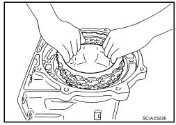
54. Remove snap ring using suitable tool.
