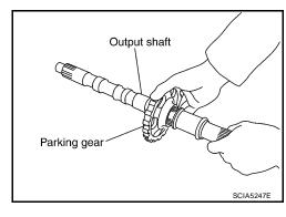
47. Remove seal rings from output shaft.
