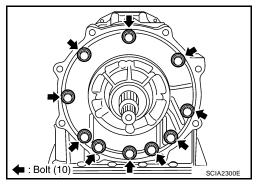
Remove the oil pump assembly evenly from the transmission case using Tools.
