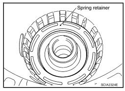
17. Install snap ring in transmission case while compressing return spring using Tool.
