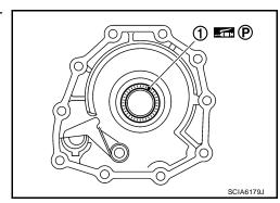
29. Install seal rings to output shaft.
