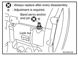
48. Install brake band in transmission case.
