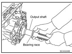
45. Remove output shaft from transmission case by rotating left/ right.
