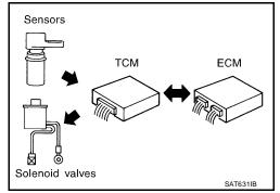
It is much more difficult to diagnose a error that occurs intermittently rather than continuously. Most intermittent errors are caused by poor electric connections or improper wiring. In this case, careful checking of suspected circuits may help prevent the replacement of good parts.
