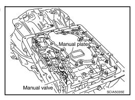
h. Install bolts A, B and C to control valve with TCM.
