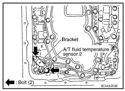
7. Remove bracket from A/T fluid temperature sensor 2.
