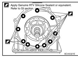
5. Tighten oil pump bolts to specified torque.
