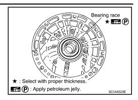
10. Remove needle bearing from front sun gear.
