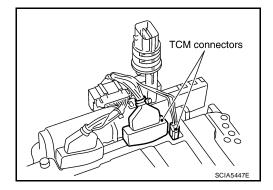
17. Remove A/T assembly harness connector from control valve with TCM using suitable tool.
