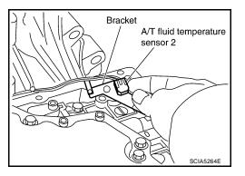
Install A/T fluid temperature sensor 2 (with bracket) in control valve with TCM. Tighten A/T fluid temperature sensor 2 bolt to the specified torque. Refer to <u>AT-233, "COMPONENTS"</u>.
