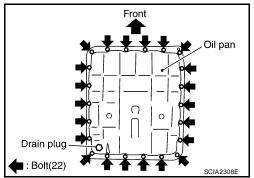
Tighten oil pan bolts to the specified torque in numerical order shown after temporarily tightening them.
