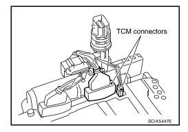
41. Remove A/T assembly harness connector from control valve with TCM using suitable tool.
