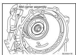
45. Install front carrier assembly, input clutch assembly and rear internal gear as a unit.
