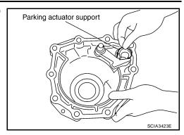
73. Remove parking pawl (with return spring) and pawl shaft from rear extension (2WD models) or adapter case (4WD models).
