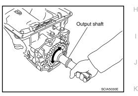
32. Install bearing race to output shaft.
