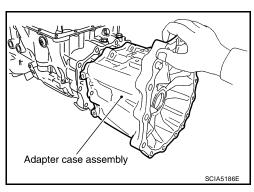
iii. Tighten adapter case assembly bolts (1) to specified torque. (With terminal bracket (2).)
