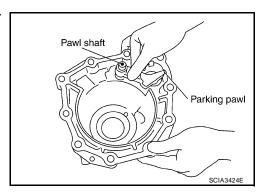
27. Install parking actuator support to rear extension (2WD models) or adapter case (4WD models).
