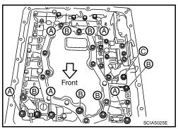
i. Tighten bolt 1, 2 and 3 temporarily to prevent dislocation. After that tighten them in order (1  $\rightarrow$  2  $\rightarrow$  3), and then tighten other bolts.
