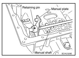
61. Remove manual shaft retaining pin with a pair of nippers.
