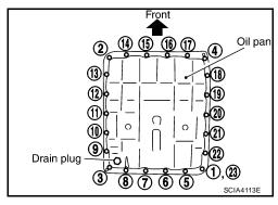
4. Install drain plug to oil pan and tighten to specification.
