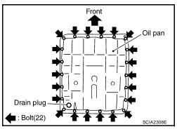
3. Check for foreign materials in oil pan to help determine cause of malfunction. If the A/T fluid is very dark, has some burned smell, or contains foreign particles then friction material (clutches, band) may need replacement. A tacky film that will not wipe clean indicates varnish build up. Varnish can cause valves, servo, and clutches to stick and can inhibit pump pressure.
