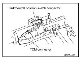
Install A/T assembly harness connector to control valve with TCM.
