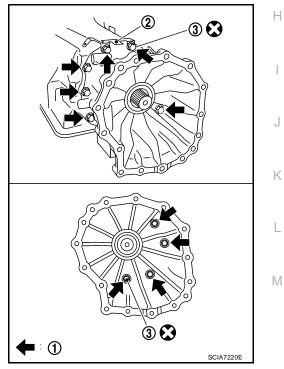
Tap adapter case assembly with soft hammer.
