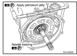
Remove front sun gear assembly from front carrier assembly.
