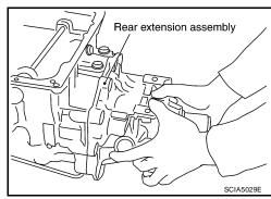
iii. Tighten rear extension assembly bolts to specified torque.
