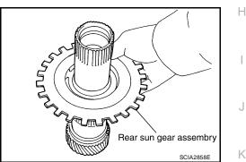
a. Remove snap ring from rear sun gear using suitable tool.
