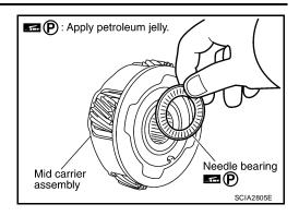
19. Remove needle bearing (rear side) from mid carrier assembly.
