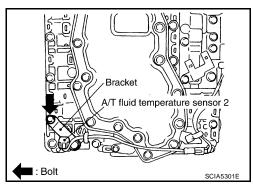
g. Install control valve with TCM in transmission case.
