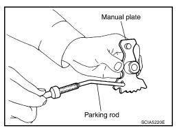
Install manual plate (with parking rod) to manual shaft.
