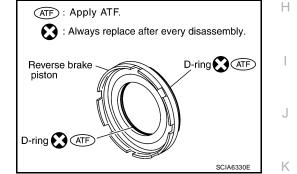
13. Install reverse brake piston in transmission case.
