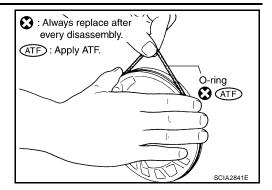
4. Remove O-ring from oil pump cover.
