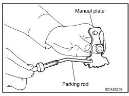
64. Remove manual shaft from transmission case.
