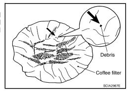
b. If one or more pieces of debris are found that are over 1mm (0.040 in) in size and/or peeled clutch facing material is found in the coffee filter, the fluid cooler is not serviceable. The A/T fluid cooler/radiator must be replaced and the inspection procedure is ended. Refer to CO-14, "RADIATOR".
