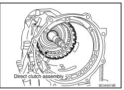
35. Install needle bearing in drum support.
