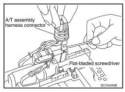
18. Disconnect TCM connector and park/neutral position switch connector
