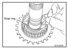
Remove high and low reverse clutch hub from mid sun gear assembly.
