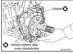
44. Remove bearing race from output shaft.
