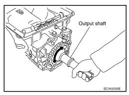
46. Remove parking gear from output shaft.
