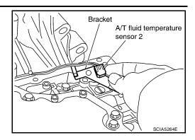
6. Install A/T fluid temperature sensor 2 (with bracket) in control valve with TCM. Tighten A/T fluid temperature sensor 2 bolt to the specified torque. Refer to AT-233, "COMPONENTS".
