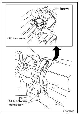
5. Remove GPS antenna and feeder assembly out the top of instrument panel.
