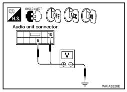
3. Check voltage between subwoofer (BOSE system) and ground.
