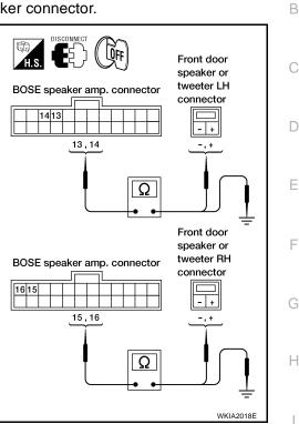
3. Check continuity between BOSE speaker amp. harness connector terminal B75 and ground.
