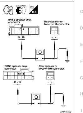
3. Check continuity between BOSE speaker amp. harness connector B75 terminal and ground.
