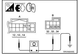
4. Check continuity between AV switch M98 (A) and ground.
