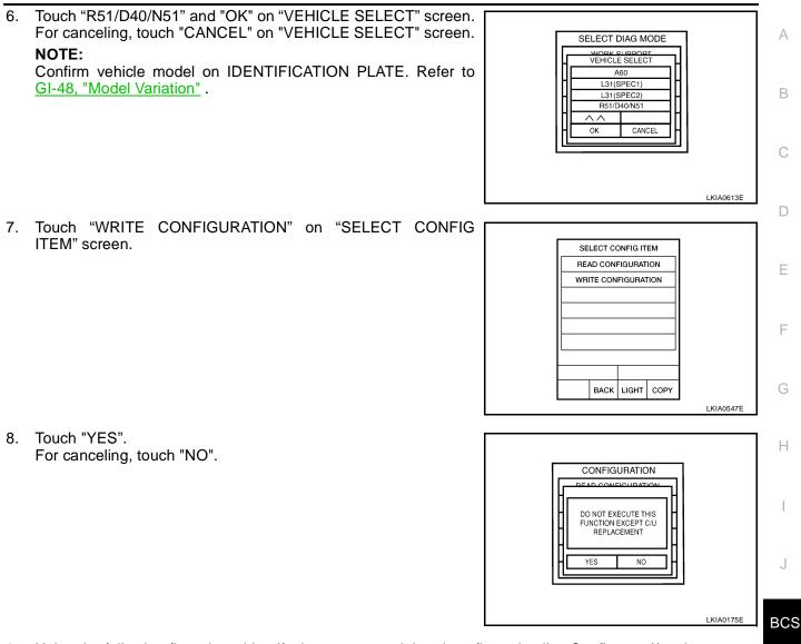
9. Using the following flow chart, identify the correct model and configuration list. Confirm and/or change setting value for each item according to the configuration list. Depending on CONSULT-II software version being used, some or all of the write configuration items shown in the following configuration lists may be displayed. If an item does not appear on the CONSULT-II "WRITE CONFIGURATION" screen(s), then it is an auto setting item and it cannot be manually set or
