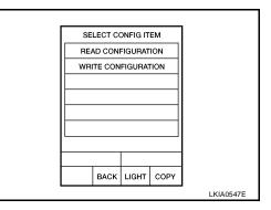
Configuration of current BCM is printed out automatically. A listing of manual setting items and auto setting items will be displayed. Auto setting items are preset and cannot be changed. Manual setting items can be set by using WRITE CONFIGURA-TION PROCEDURE. Refer to <u>BCS-23</u>, "WRITE CONFIGURA-<u>TION PROCEDURE"</u>.
