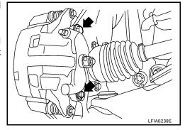
Install brake hose to cylinder body, if removed, then tighten union bolt to the specified torque. Refer to <u>BR-24</u>, "Components".
