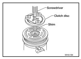
Install the clutch pulley bolt using Tool, to prevent the clutch disc from turning and tighten the bolt to specification. Refer to <u>MTC-101, "COMPONENTS"</u>.
