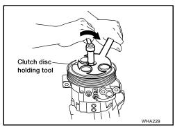
Check the pulley clearance all the way around the clutch disc as shown.
