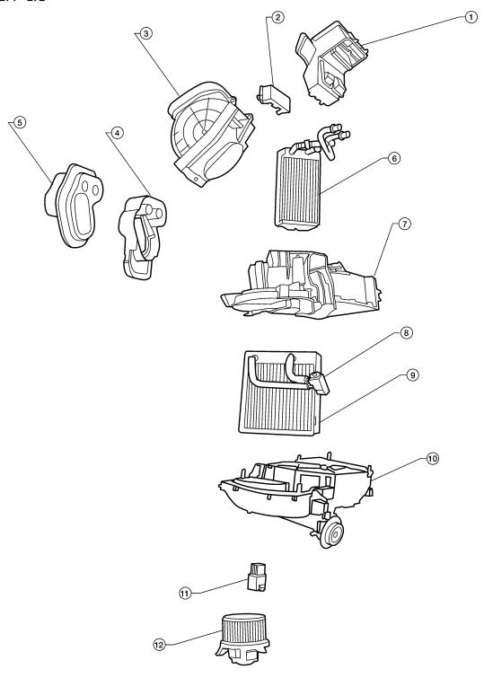
Center ventilator connector duct 2. Intake air case 1. Front heater core cover 3. Α Front heater core and evaporator Front heater core and evaporator 6. Front heater core pipes bracket pipes grommet Upper heater and cooling unit case Front expansion valve 9. Front evaporator 7. 8. В 10. Lower heater and cooling unit case 11. Variable blower control 12. Blower motor
