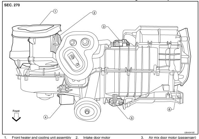
Front heater and cooling unit assembly
