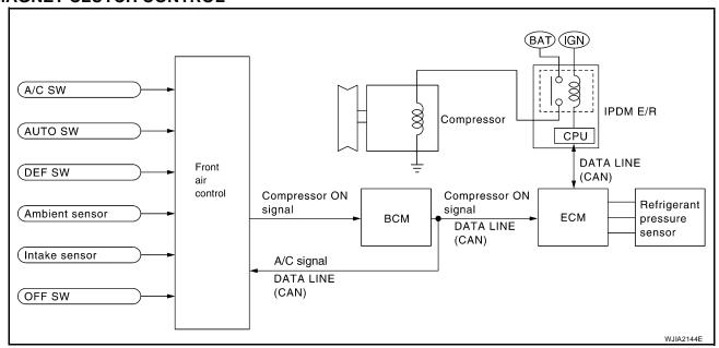
When A/C switch or DEF switch is pressed, front air control inputs compressor ON signal to BCM.
