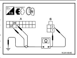
4. Check continuity between optical sensor harness connector M145 (B) terminal 1 and 2 and ground.
