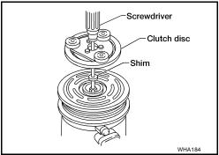
5. Install the clutch pulley bolt using Tool, to prevent the clutch disc from turning and tighten the bolt to specification. Refer to <a href="ATC-160">ATC-160</a>, "Components".
