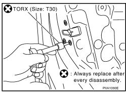
8. While pulling outside handle bracket, slide toward rear of vehicle to remove outside handle bracket and door lock assembly.
