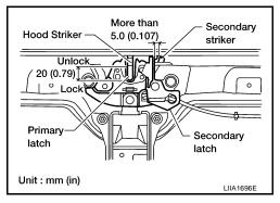
After adjusting hood lock, tighten the lock bolts to the specified torque.
