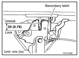
4. Check the hood lock lubrication condition. If necessary, apply "body grease" to the points shown.
