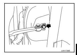
Remove the door-side hinge nuts, and remove the door assembly.
