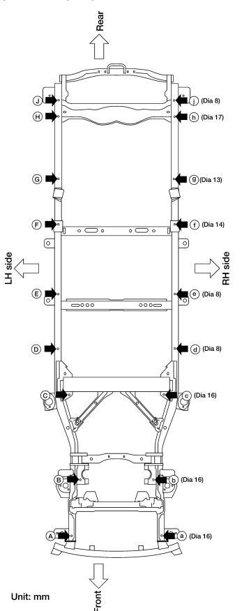
Coordinates: (A)(a) X: ± 425 Y:-531 Z: 275 B,bX: ± 353 Y:35 Z:304 ©.© X: ± 460 Y:807 Z:100  $\bigcirc$  d X: ± 568 Y:1356 Z:109 E,e X: ± 570 Y:1710 Z:99 (F)(f)X: ± 555 Y:2420 Z:205 GgX: ± 559 Y:3066 Z:400 H)h X: ± 559 Y: 3471 Z:400 **J**,(j) X: ± 560 Y:3652 Z:368
