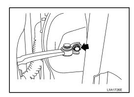
Remove the door-side hinge nuts, and the door assembly.
