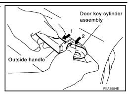
5. While pulling outside handle, slide toward rear of vehicle to remove outside handle.
