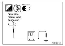
3. Check continuity between front parking lamp harness connector and ground.
