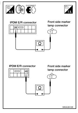
Check continuity between IPDM E/R harness connector and front parking lamp harness connector.
