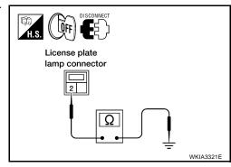
Check continuity between rear combination lamp harness connector and ground.
