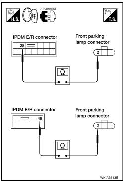
5. Check continuity between IPDM E/R harness connector and license plate lamp harness connector.
