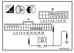
4. Check for continuity between each terminal of BCM harness connector in suspect malfunctioning system and ground.
