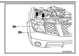
4. Disconnect the front combination lamp connector and remove front combination lamp.
