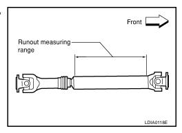
While holding the flange yoke on one side, check axial play of the joint as shown. If the journal axial play exceeds the specification, repair or replace the journal parts.
