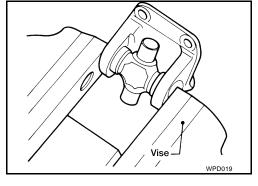
2. Select new snap rings that will provide the specified play in an axial direction of the journal, and install them. Refer to PR-15, "Snap Ring".
