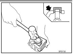
4. Push out and remove the remaining journal bearings at the opposite side by lightly tapping the flange yoke with a hammer, taking care not to damage the journal or flange yoke hole.
