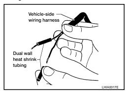
5. Fold each wire back and insert into the end of the heat shrink tubing so that the end of the wire is approximately centered in the heat shrink tubing.
