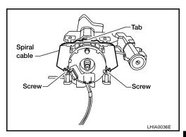
8. Disconnect the spiral cable connectors.
