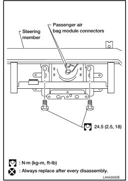
6. Remove front passenger air bag module screws then remove passenger air bag module from instrument panel assembly.
