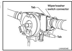
Disconnect lighting and turn signal switch connector. Then while pressing tabs, pull lighting and turn signal switch toward driver door to remove.
