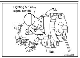
7. Remove the screws. Then while pressing the tab, pull the spiral cable away from steering column assembly.
