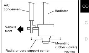
b. Lift A/C condenser up and remove radiator after disengaging the fitting at front-bottom surface.
