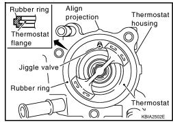
Installation of Water Outlet Pipe and Heater Pipe
