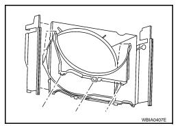
8. Remove the upper radiator shroud upper bolts and remove the upper radiator shroud (A).
