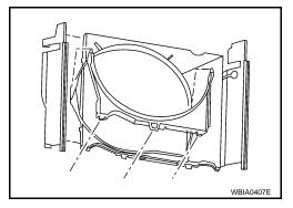
9. Remove the radiator shroud (upper) bolts and remove the radiator shroud (upper) (A).
