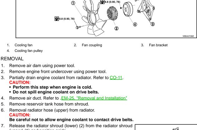
(upper) (1) and position aside.Release the tabs, pull radiator shroud (lower) (2) rearwards and down.
