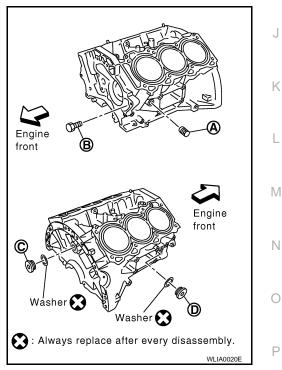
Block Plug and Block Heater Installation
