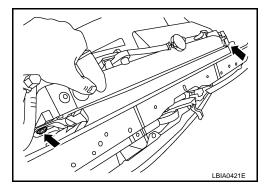
12. Remove the two A/C condenser bolts.
