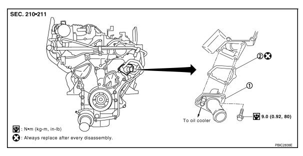
1. Water inlet and thermostat assembly 2. Gasket
