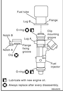
4. Install the fuel tube and fuel injector assembly to the intake manifold. CAUTION:
