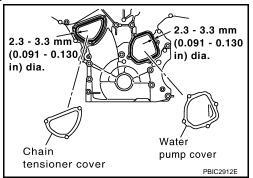
4. Install front timing chain case as follows:
