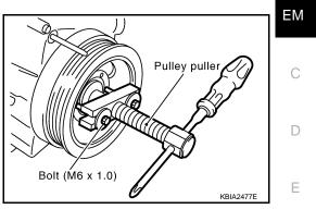
7. Remove the front oil seal using suitable tool. CAUTION: Do not damage front cover and oil pump drive spacer.
