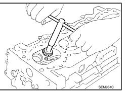
6. Using compound, grind to adjust valve fitting.
