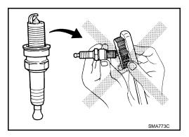
• If plug tip is covered with carbon, spark plug cleaner may be used.
