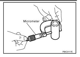
Connecting Rod Bushing Oil Clearance (Small End)
