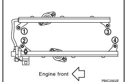
6. Remove bolts which connects fuel tube (RH) and fuel tube (LH).
