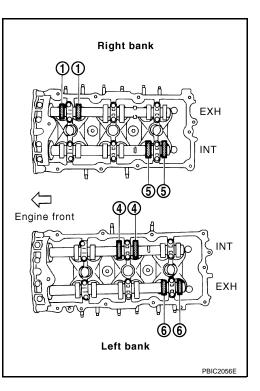
4. For the measured value out of the standard, perform adjustment.
