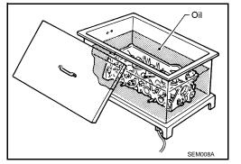
Heat cylinder head to 110° to 130°C (230° to 266°F) by soaking in heated oil.
