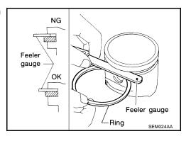
• If the measured value exceeds the limit, replace piston ring, and measure again. If it still exceeds the limit, replace piston also.
