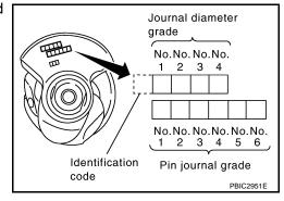
When Crankshaft and Connecting Rod are Reused
