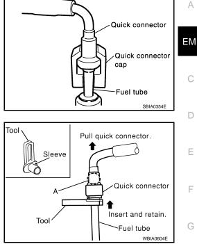
With the sleeve side of Tool facing quick connector, install Tool onto fuel tube.
