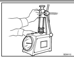
• If measurement is not within specifications, replace the valve spring.
