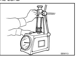
• If the installation load or load with valve open is out of the standard, replace valve spring.
