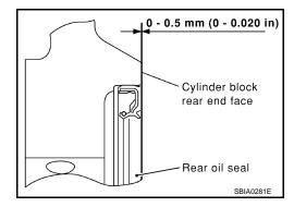
• Press in rear oil seal to the position as shown.
