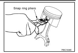
b. Heat piston to  $60^\circ$  to  $70^\circ C$  (140° to 158°F) with industrial use drier or equivalent.
