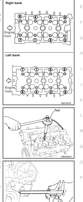
After installing cylinder head, measure distance between front 4. end faces of cylinder block and cylinder head (left and right banks).
