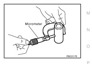
Piston to Piston Pin Clearance
