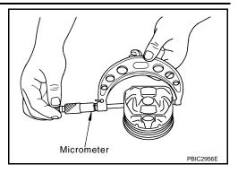
Piston to Cylinder Bore Clearance
