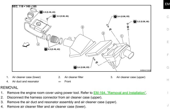
Add marks as necessary for easier installation.
