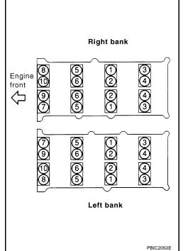
6. Measure the difference in levels between front end faces of camshaft bracket (No. 1) and cylinder head.
