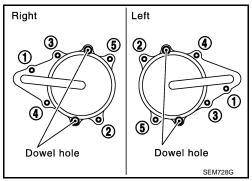
13. Remove collared O-rings from front timing chain case (left and right side).
