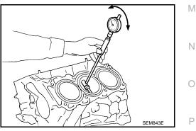
MAIN BEARING HOUSING INNER DIAMETER
