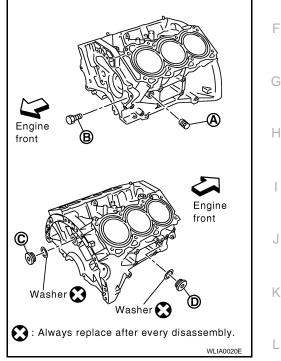
Tighten each plug as specified below.
