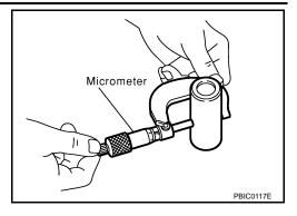
Piston to Piston Pin Oil Clearance
