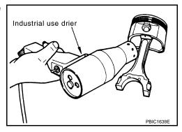
c. Push out piston pin with stick of outer diameter approximately 20 mm (0.79 in).
