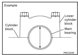
If the calculated value exceeds the limit, select proper main bearing according to main bearing inner diameter and crankshaft main journal diameter to obtain specified bearing oil clearance. Refer to <u>EM-127</u>, "<u>How to</u> <u>Select Piston and Bearing</u>".
