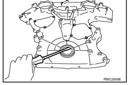
22. Use a scraper to remove all traces of old liquid gasket from front and rear timing chain cases and oil pan (upper), and liquid gasket mating surfaces. CAUTION:
