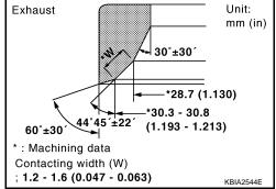
7. Check again for normal contact. Follow the "VALVE SEAT CONTACT" procedure.
