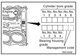
When Cylinder Block is Reused
