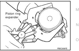
16. Remove piston from connecting rod as follows:
