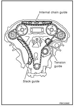
Remove timing chain (primary) and crankshaft sprocket.
