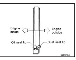
• Install new rear oil seal using Tool.
