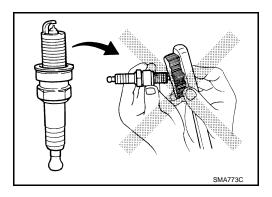
• If the spark plug tip is covered with carbon, a spark plug cleaner may be used.
