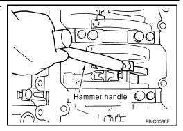
Remove connecting rod bearings.
