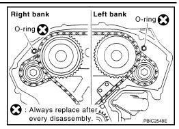
Fit lower end of front timing chain case tightly onto top face of oil pan (upper). From the fitting point, make entire front timing chain Front timing chain case Engine front Cylinder block Oil pan (upper) PBIC1100E
