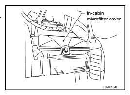
Insert the first new in-cabin microfilter into the front heater and cooling unit housing and slide it over to the right. Insert the second new in-cabin microfilter into the front heater and cooling unit housing.
