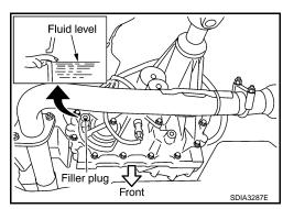
3. Install the filler plug with a new gasket to the transfer. Tighten to the specified torque. Refer to <u>DLN-149</u>. "Disassembly and Assembly" (ATX14B), DLN-288, "Disassembly and Assembly" (TX15B).
