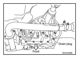
Install the drain plug with a new gasket to the transfer. Tighten to the specified torque. Refer to <u>DLN-149</u>, "<u>Disassembly and Assembly</u>" (ATX14B), <u>DLN-288</u>, "<u>Disassembly and Assembly</u>" (TX15B).
