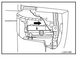
5. Install the in-cabin microfilter cover.
