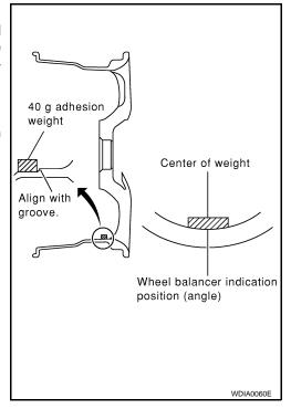
If calculated balance weight value exceeds 50 g (1.76 oz), install two balance weight sheets in line with each other as shown.
