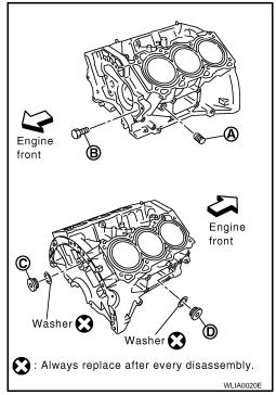
Block Plug and Block Heater Installation
