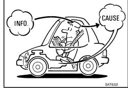
Before undertaking actual checks, take a few minutes to talk with a customer who approaches with a driveability complaint. The customer can supply good information about such errors, especially intermittent ones. Find out what symptoms are present and under what conditions they occur. A "Diagnostic work sheet" as shown on the example (Refer to TM-7) should be used.
