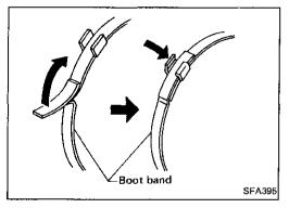
7. Lock new larger and smaller boot bands securely with a suitable tool.
