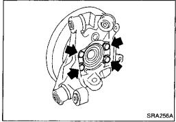
Remove wheel bearing with flange, and wheel hub from axle housing.
