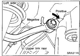
If camber is not within specification, adjust by turning the adjusting bolt.
