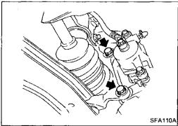
Remove brake caliper assembly.
