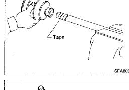
Set joint assembly onto drive shaft by lightly tapping it. Install joint assembly securely, ensuring marks which were made during disassembly are properly aligned.
