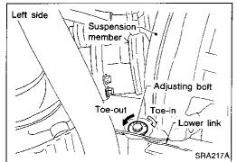
Adjust toe-in by turning adjusting bolts. For models equipped with SUPER HICAS system, refer to SUPER HICAS in ST section.
