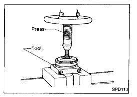
5. Remove center bearing with Tool and press. Tool number: \$T30031000 (J22912-01)
