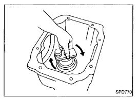
Install the pinion rear bearing inner cone into the final drive 3. PD housing. Then place the pinion preload shim selector Tool
