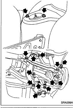
• Retighten all nuts and bolts to the specified torque.
