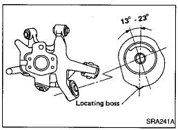
When installing shock absorber bushing, make sure that it is positioned as shown.
