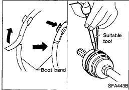
Lock new larger and smaller boot bands securely with a suitable tool.
