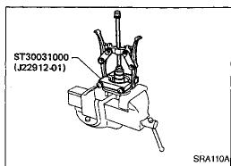
Remove inner race from hub using a bearing replacer/ puller.
