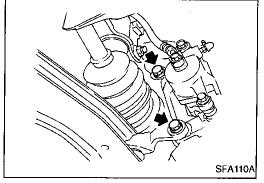
Remove brake caliper assembly and rotor.
