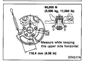
With wheel hub pressed into axle housing, apply 49,000 N (5,000 kg, 11,000 lb) to wheel hub and rotate both clockwise and counterclockwise 10 times to minimize resistance.
