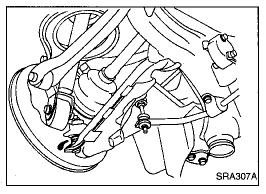
Check suspension ball joint for grease leakage and ball joint dust cover for cracks or other damage.
