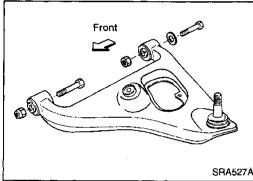
Before removing, put matchmarks on adjusting bolt.
