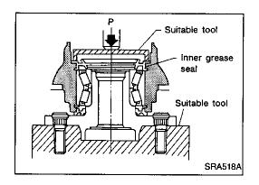
Install inner grease seal.
