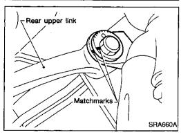
When installing, final tightening must be done under unladen condition with tires on ground.
