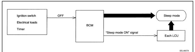
"Sleep" control prevents unnecessary power consumption. After the following conditions are met, the BCM suspends the communication between itself and all LCUs. The whole IVMS is set in the "sleep" mode.
