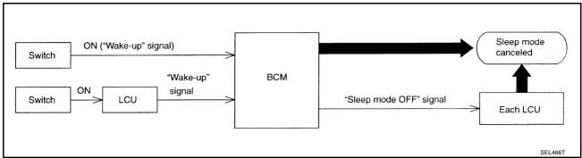
As shown above, when the BCM detects a "wake-up" signal, it wakes up the whole system and starts communicating again. The "sleep" mode of all LCUs is now canceled, and the BCM returns to the normal control mode. When any one of the following switches are turned ON, the "sleep" mode is canceled:
