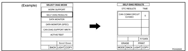
Print all the data of "CAN DIAG SUPPORT MNTR" for "ENGINE", "VDC", "ICC", and "A/T" displayed on CONSULT-II.
