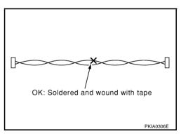
Do not perform bypass wire connections for the repair parts.
