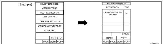
2. Print all the data of "CAN DIAG SUPPORT MNTR" for "ENGINE", "VDC", and "A/T" displayed on CON-SULT-II.
