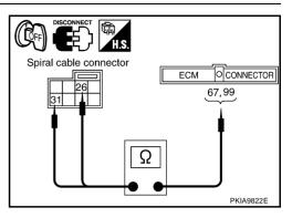
4. Check continuity between spiral cable harness connector M53 terminals 31 (B), 26(G/OR) and ground.
