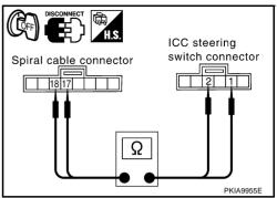
2. Check continuity between spiral cable harness connector M441 terminals 18 (Y), 17 (G) and ground.
