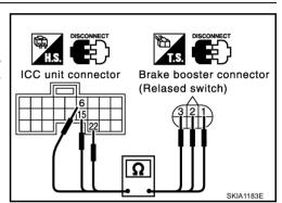
4. Check continuity between ICC unit harness connector B243 terminals 6 (L), 15 (P), 22 (R/B) and ground.
