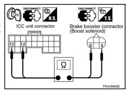
Check continuity between ICC unit harness connector B243 terminals 10 (W/R), 12 (B/R) and ground.
