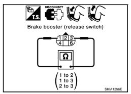
(Note): However, if pedal is depressed insufficiently, resistance value may remain unchanged.
