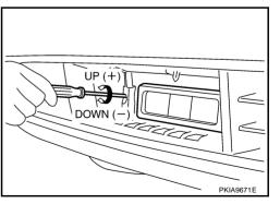
When "U/D CORRECT" value indicates ±4, confirm that the margin of value remains within ±4 at least for 2 seconds with no equipment or hand touching the ICC sensor.
