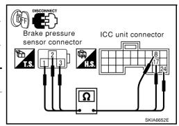
Check continuity between ICC unit harness connector and ground.
