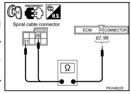
4. Check continuity between spiral cable harness connector and ground.
