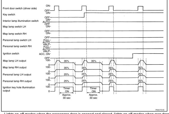
Lights on-off modes when the passenger door is opened and closed, lights on-off modes when rear doors (LH, RH) are opened and closed.
