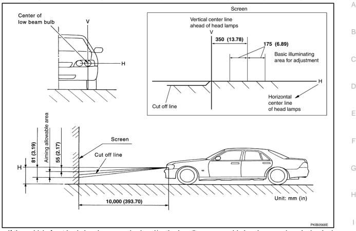
If the vehicle front body has been repaired and/or the headlamp assembly has been replaced, check aiming. Use the aiming chart shown in the figure.
