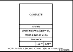
3. Touch "IVMS" on "SELECT SYSTEM" screen. If "IVMS" is not indicated, refer to <u>GI-37, "CONSULT-II Data Link Connector</u> (<u>DLC) Circuit</u>".
