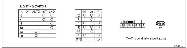
Hi: "HIGH BEAM" position, Lo: "LOW BEAM" position, P: "FLASH TO PASS" position
