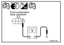
5. Check voltage between front combination lamp harness connector terminal 9 and ground for each of UP, MID, and DOWN active test positions.
