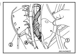
e. Apply a strip of protective tape (A) on body panel to protect it from damage.
