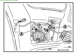
3. Remove harness protector ①, and then remove front turn signal lamp assembly ② from front bumper fascia.
