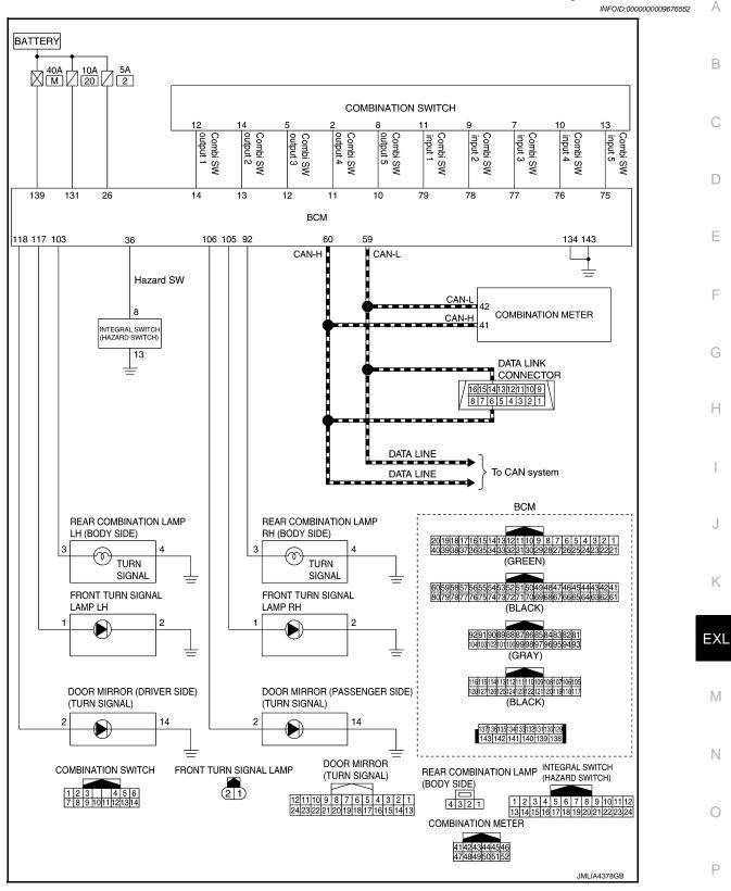
PARKING, LICENSE PLATE, SIDE MARKER AND TAIL LAMP SYSTEM PARKING, LICENSE PLATE, SIDE MARKER AND TAIL LAMP SYSTEM : System De-
