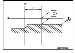
Adjust the cutoff line height (X) with the aiming adjustment screw so as to enter in the adjustment range (M–N) according to the horizontal center line of headlamp (H).
