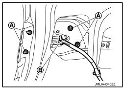
Pull rear combination lamp (trunk lid side) out off trunk lid panel and remove it.
