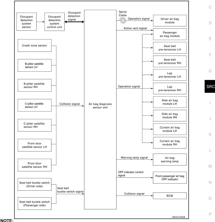
For models for Mexico, front door satellite sensors and active vent signal are not applied.
