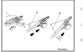
3. Replace the seat belt assembly if it does not operate normally.
