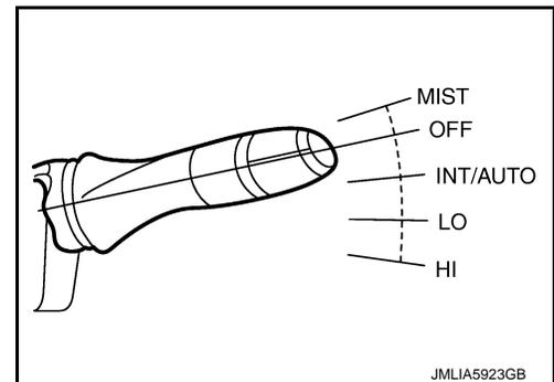
4. To exit service position, turn ignition switch ON and operate front wiper switch.
