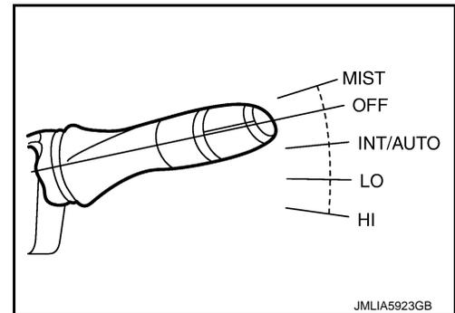
5. To exit service position, operate front wiper switch.
