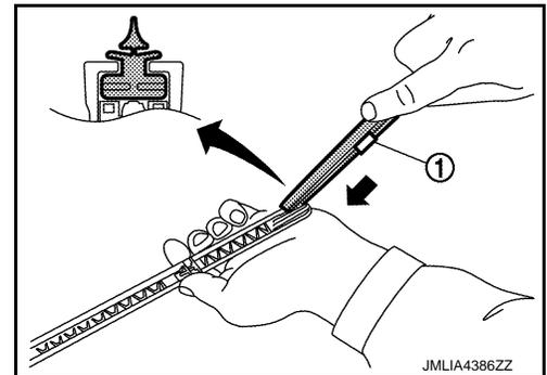
3. Engage wiper refill stopper hole, and wiper blade pawl with imprinted "SET" mark ("←" mark).
