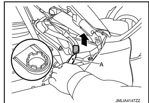
3. Remove wiper arm fixing nut, and then remove wiper arm.
