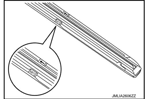
2. Pass through pawl of wiper blade in the groove of wiper refill.
