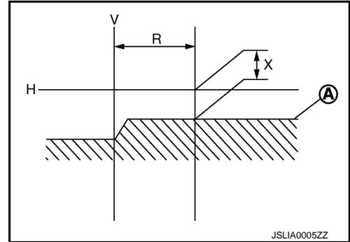
5. Adjust the cutoff line height (X) with the aiming adjustment screw so as to enter in the adjustment range (M–N) according to the horizontal center line of headlamp (H).
