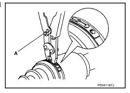
• Secure boot band so that dimension (M) meets the specification as shown in the figure.
