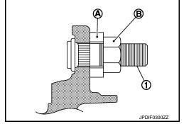
Clean the matching surface of drive shaft and wheel hub and bearing assembly. And then apply paste [service parts (440037S000)] to surface (A) of joint sub-assembly of drive shaft.
