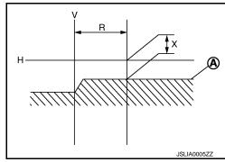
Adjust the cutoff line height (X) with the aiming adjustment screw so as to enter in the adjustment range (M–N) according to the horizontal center line of headlamp (H).
