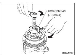
Remove the clutch disc using the clutch disc puller.
