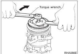
Using the holder to prevent clutch disc rotation, tighten the bolt to 14 N·m (1.4 kg-m, 10 ft-lb) torque. After tightening the bolt, check that the pulley rotates smoothly.
