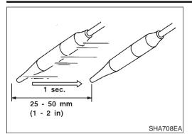
Move probe along component approximately 25 to 50 mm (1 to 2 in)/sec.
