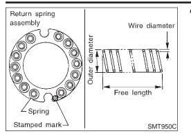
• Check stamped mark shown in the figure. Then, check that free length, outer diameter and wire diameter are within specifications. If any abnormality is found, replace with new return spring assembly of the same stamped number.
