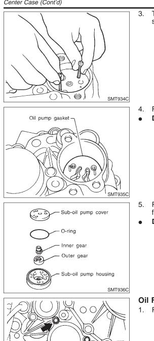
Thread two bolts (M4 x 0.8) into the holes of sub-oil pump as shown in the figure, and pull out to remove sub-oil pump.
