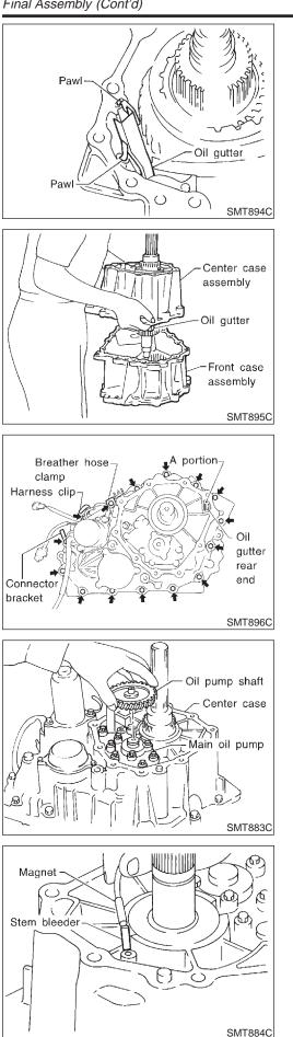
4. Make sure the two claws of oil gutter are securely attached to slots in center case.
