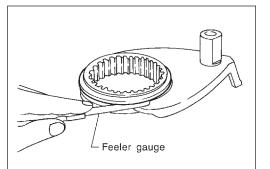
• Measure clearance between shift fork and sleeve. If it is out of specification, replace it with new one.
