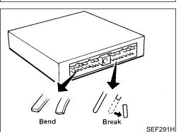
When connecting or disconnecting pin connectors into or SC from Transfer control unit, take care not to damage pin terminals (bend or break). Make sure that there are not any bends or breaks on EL Transfer control unit pin terminal, when connecting pin connectors.
