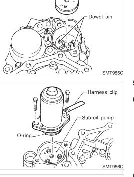
4. Align dowel pin hole and mounting bolt hole of sub-oil pump assembly with center case. Then tighten bolts.
