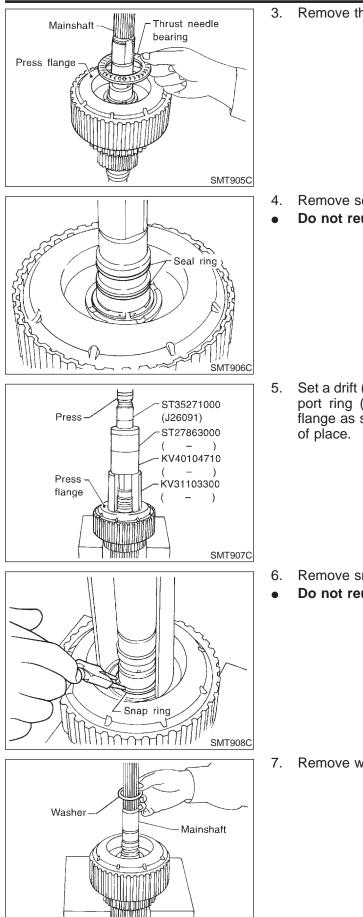
Remove thrust needle bearing from press flange.
